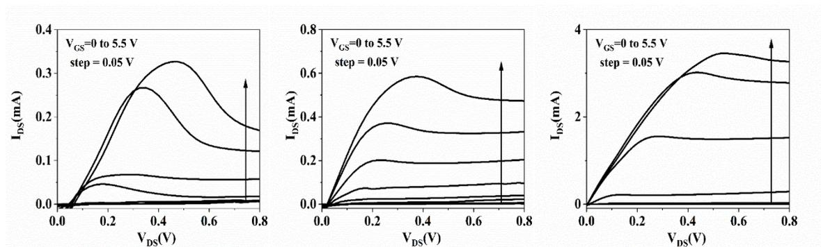
**Figure S8.** Output curves of OECTs based on P-AQM2I-2T, P-AQM2I-TT and P-AQM2I-2T.
