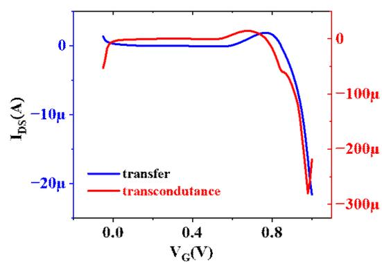
**Figure S9.** Transfer and normalized transconductance curves of OEETs based on P-AQM2I-2T with a  $V_{DS}$  of 0.3 V after annealing at 100 ° C for 10 min.
