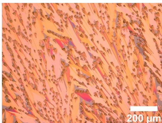
**Figure S71** Reflection polarized light micrograph from dip coated film of **3n-Cl** on CDPA-modified  $\text{AlO}_x/\text{SiO}_2$  using  $\text{CH}_2\text{Cl}_2/\text{Acetone}$  as solvent.
