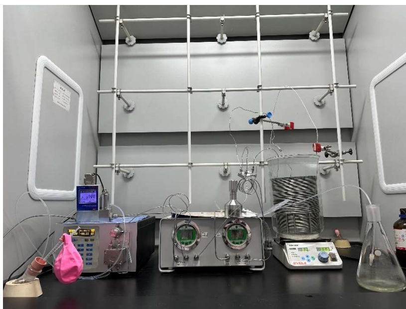
Figure S2 Set-up for asymmetric hydrogenation under continuous flow.
