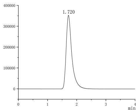
**Figure S7.** GC of H<sub>2</sub> standard sample
