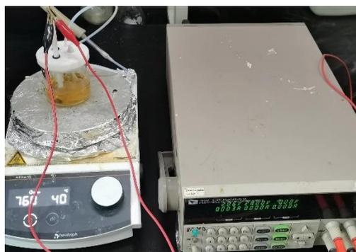
**Figure S7.** The ElectraSyn Set-up.
