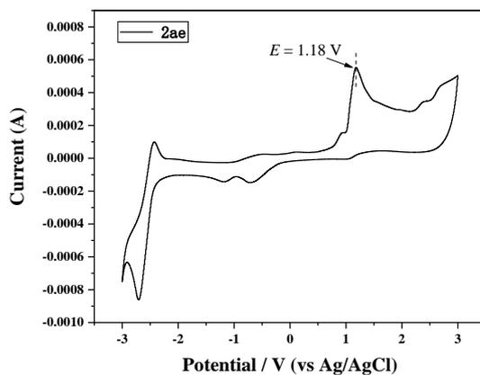
**Figure S2.** Cyclic voltammogram of **2ae** (0.01 M) in an electrolyte of  $n\text{Bu}_4\text{NBF}_4$  (0.1 M) in  $\text{CH}_3\text{CN}$ .  $E = 1.18$  V.
