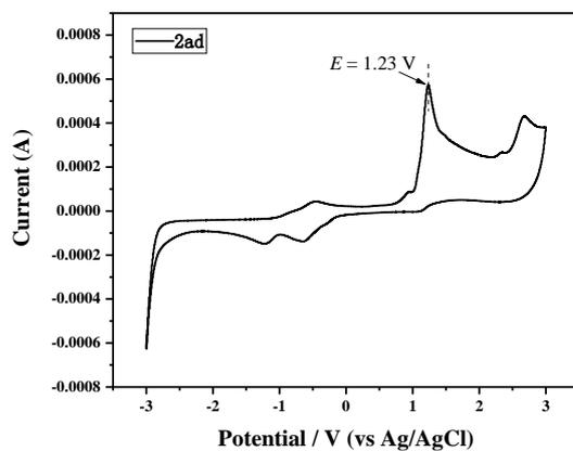
**Figure S1.** Cyclic voltammogram of **2ad** (0.01 M) in an electrolyte of  $n\text{Bu}_4\text{NBF}_4$  (0.1 M) in  $\text{CH}_3\text{CN}$ .  $E = 1.23$  V.
