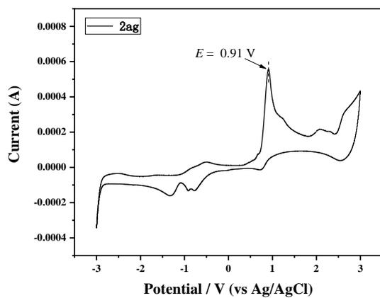
**Figure S4.** Cyclic voltammogram of **2ag** (0.01 M) in an electrolyte of  $n\text{Bu}_4\text{NBF}_4$  (0.1 M) in  $\text{CH}_3\text{CN}$ .  $E = 0.91$  V.
