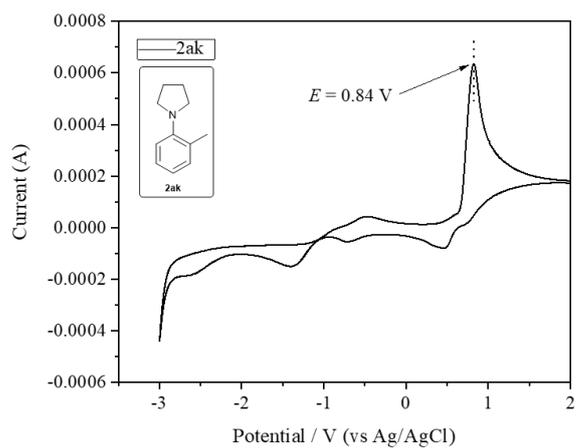
**Figure S5.** Cyclic voltammogram of **2ak** (0.01 M) in an electrolyte of  $n\text{Bu}_4\text{NBF}_4$  (0.1 M) in  $\text{CH}_3\text{CN}$ .  $E = 0.84$  V.
