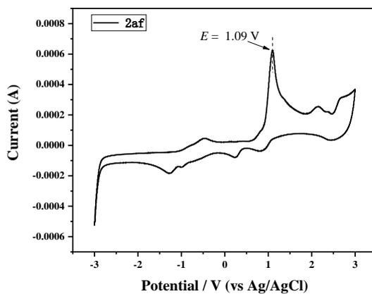
**Figure S3.** Cyclic voltammogram of **2af** (0.01 M) in an electrolyte of  $n\text{Bu}_4\text{NBF}_4$  (0.1 M) in  $\text{CH}_3\text{CN}$ .  $E = 1.09$  V.
