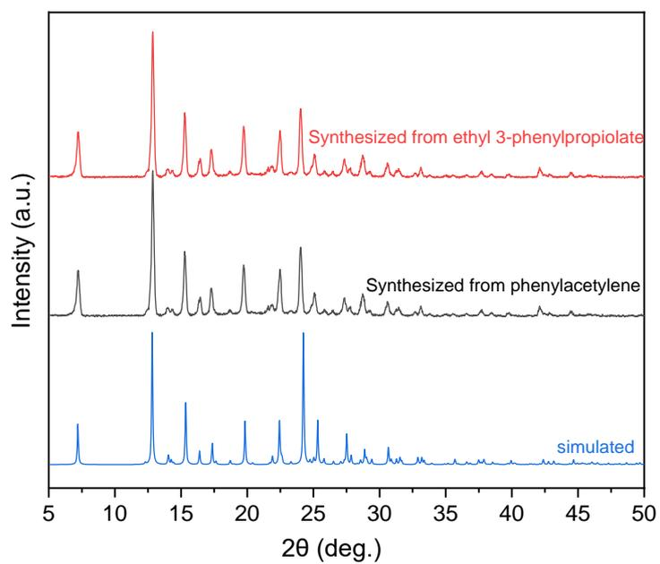
Fig S10. Experimental and simulated XRD patterns of **4d**.
