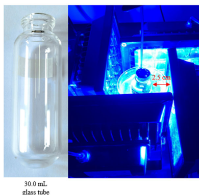
Supplementary Figure 17. Experimental setup for Gram-Scale Synthesis of Compound 3
