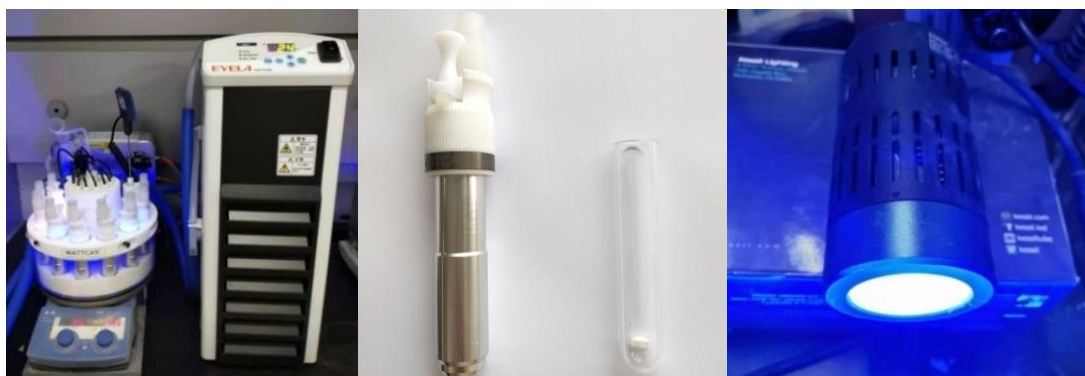
Figure S1. Instruments for photochemical reactions (5w white and blue LEDs and 40w blue LED).
