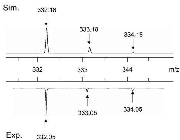
**Figure R47.** ESI-MS and isotopic pattern of **9c** indicated a charge ion  $[\mathbf{9c} + \text{H}]^+$ .
