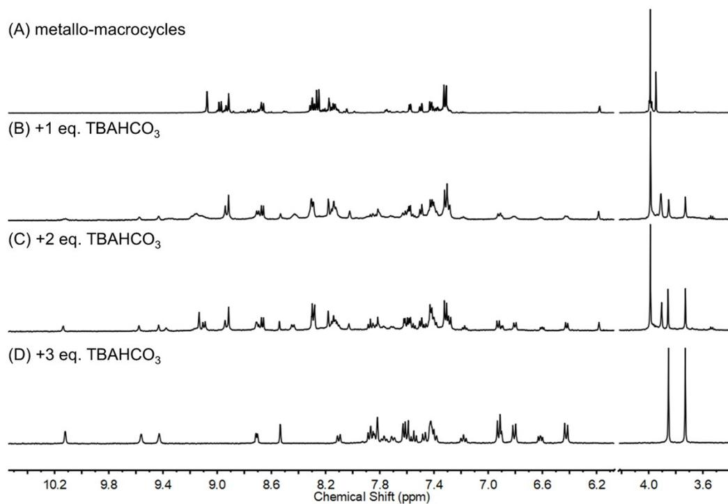
**Figure S38.**  $^1\text{H}$  NMR spectra (400 MHz,  $\text{CD}_3\text{CN-d}_3$ , 298 K) showing the conversion of a library of metallo-macrocycles to quadruple stranded helicate **D**- $\text{HCO}_3^-$  upon addition of tetrabutylammonium hydrogen carbonate: (A) a library of metallo-macrocycles, addition of (B) 1.0 equiv. of tetrabutylammonium hydrogen carbonate; (C) 2.0 equiv. of tetrabutylammonium hydrogen carbonate; (D) 3.0 equiv. of tetrabutylammonium hydrogen carbonate.
