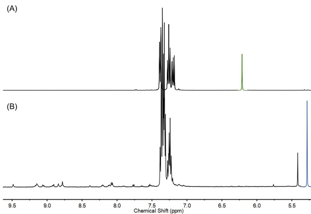
**Figure S40.** Partial  $^1\text{H}$  NMR (400 MHz, 298 K,  $\text{CDCl}_3$ ) spectrum of: (A) bromodiphenylmethane **3**; (B) The reaction mixture of 9  $\mu\text{mol}$  of **3** in presence of 10 mol% of the library (0.9  $\mu\text{mol}$ ) and 0.09 mmol  $\text{CH}_3\text{OH}$  in 0.5 mL of  $\text{CD}_3\text{CN}$  after stirring for 1 h at 40  $^\circ\text{C}$ .
