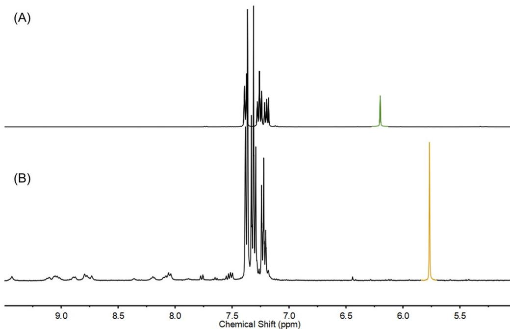
**Figure S39.** Partial  $^1\text{H}$  NMR (400 MHz, 298 K,  $\text{CDCl}_3$ ) spectrum of: (a) bromodiphenylmethane **3**; (b) The reaction mixture of 9  $\mu\text{mol}$  of **3** in presence of 10 mol% of the library (0.9  $\mu\text{mol}$ ) and 0.09 mmol  $\text{H}_2\text{O}$  in 0.5 mL of  $\text{CH}_3\text{CN}$  after stirring for 1 h at 40 °C.
