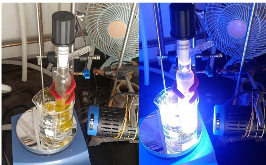
Figure S2. Reaction setup under blue LED (40 w) irradiation for gram synthesis
