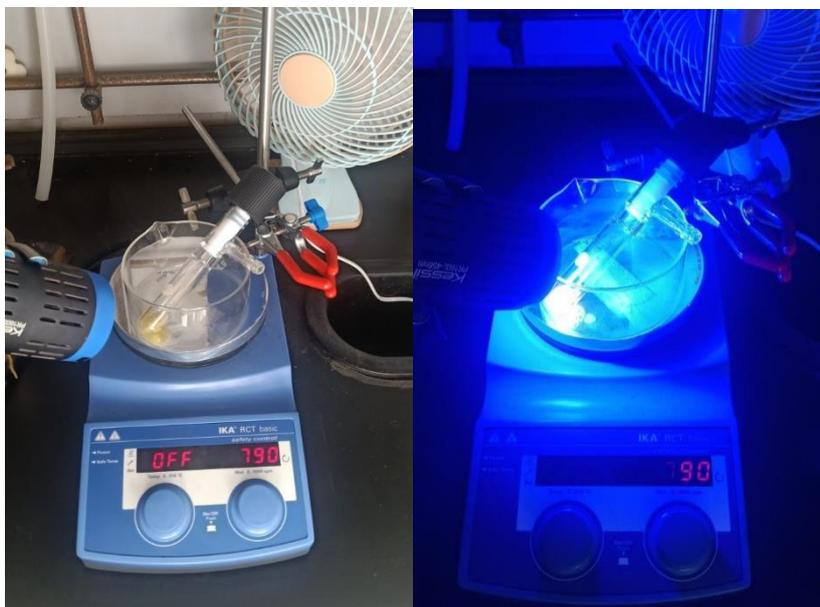
Figure S1. Reaction setup under blue LED (40 w) irradiation
