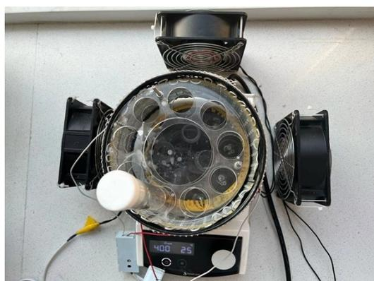
**Figure S1** Picture of DIY photocatalysis setup
