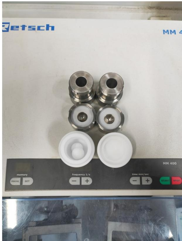
**Figure S1.** Retsch MM 400, stainless jars and balls, and PTFE-coated jars and balls were used in this study.
