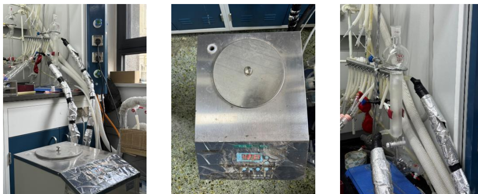
Figure S1 Column chromatography at -20 °C
