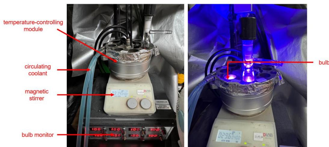
**Fig. S1** Photos of the photoreactor
