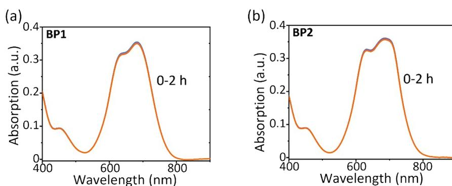
**Figure S5.** Absorption variation of (a) **BP1-NP** and (b) **BP2-NP** in PBS buffer with  $\text{H}_2\text{O}_2$  ( $100 \mu\text{M}$ ) during 2 h (interval 30 min,  $c = 10 \mu\text{M}$ )
