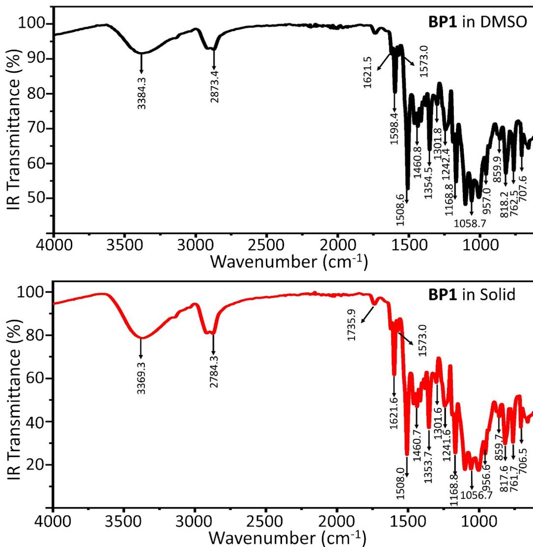
**Figure S12.** FTIR spectra of compound **BP1** at monomer (black line, in DMSO) and solid (red line) state.
