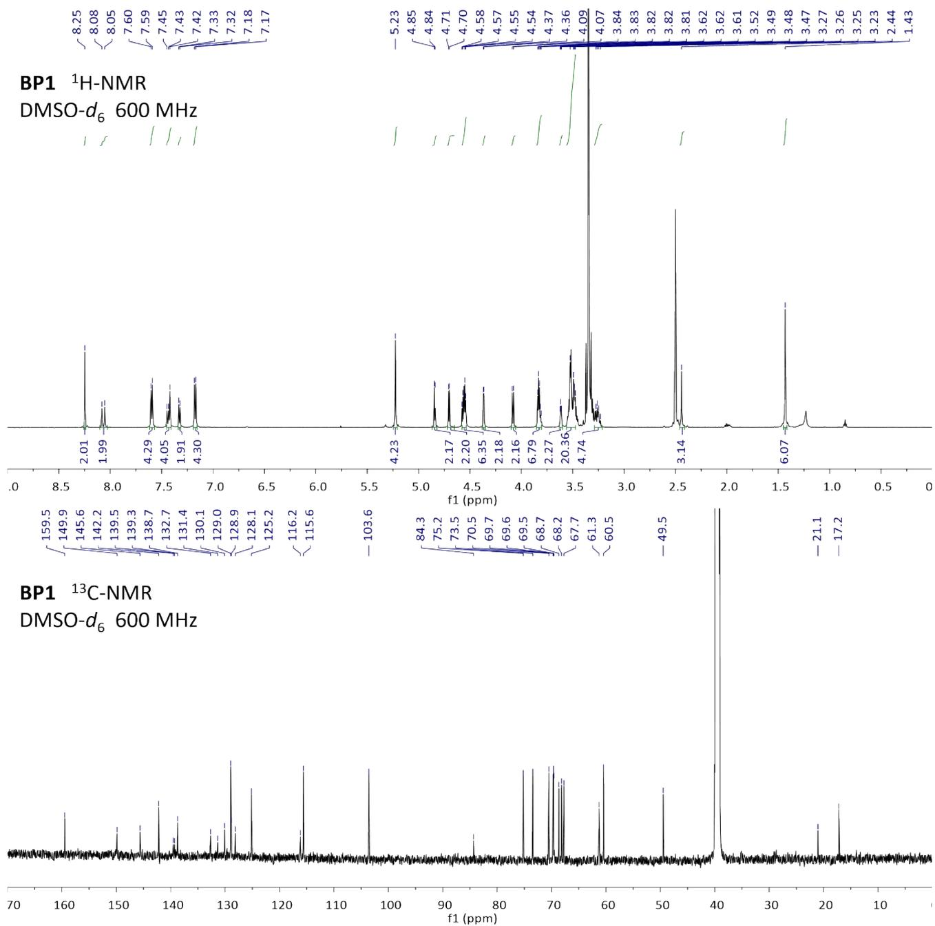
**Figure S10.**  $^1\text{H-NMR}$  and  $^{13}\text{C-NMR}$  spectra of compound **BP1** in DMSO- $d_6$ .
