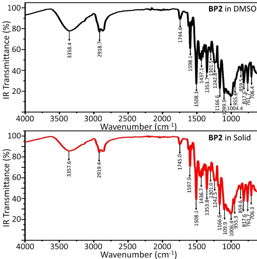
**Figure S13.** FTIR spectra of compound **BP2** at monomer (black line, in DMSO) and solid (red line) state.
