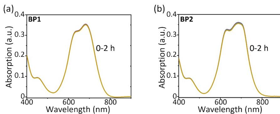
**Figure S4.** Absorption variation of (a) **BP1-NP** and (b) **BP2-NP** in PBS buffer exposed under 660 nm LED light irradiation ( $P = 50 \text{ mW cm}^{-2}$ ) during 2 h (interval 20 min,  $c = 10 \mu\text{M}$ )
