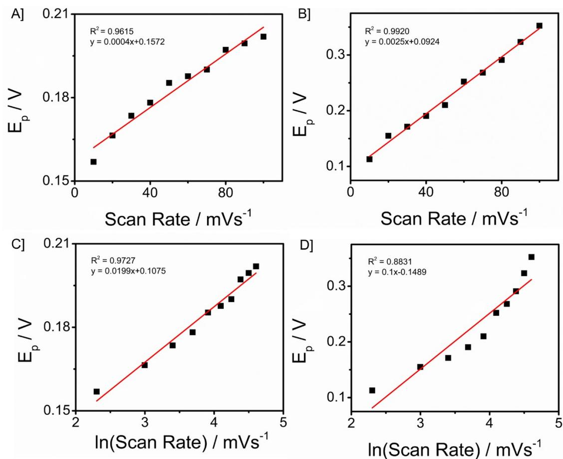
Figure S8: A] Plot of peak potential vs scan rate for 50  $\mu\text{M}$  DA in, C] Calibration plot of peak potential Vs  $\ln$  of scan rate of PBS CP/ $\text{Fe}_3\text{O}_4$ -GO/Chi electrode, B] Calibration plot of peak potential Vs scan rate and D] Peak potential Vs  $\ln$ (Scan rate) in PBS containing 50  $\mu\text{M}$  of working electrode modified with GO.
