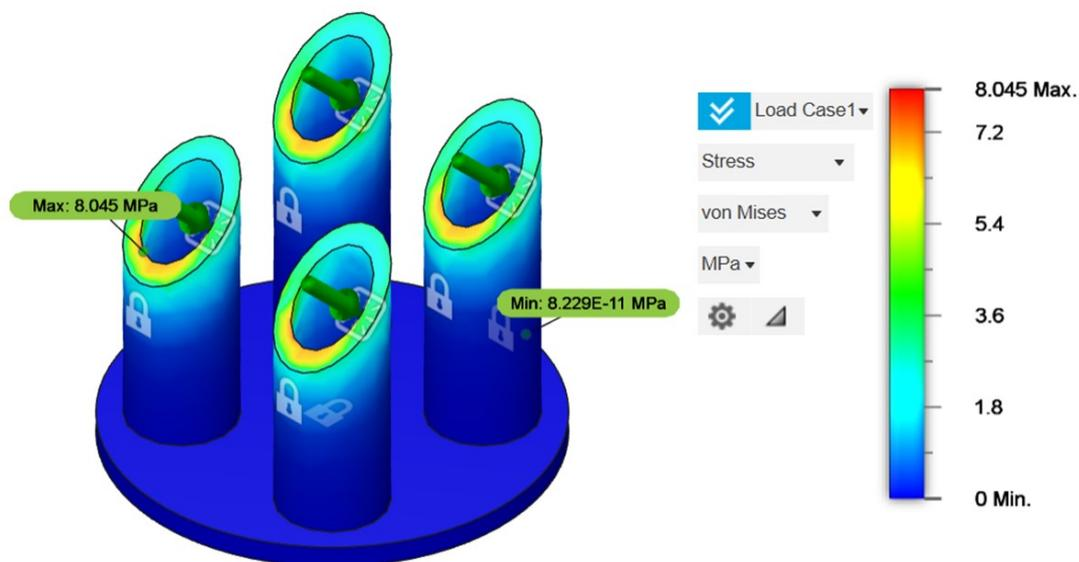
Figure S2: Microneedle insertion force analysis using the Fusion 360 simulation approach.
