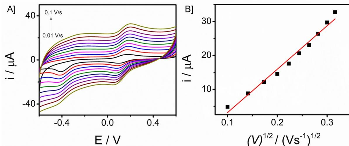
Figure S7: A] CV responses of Scan rate (0.01 V/s to 0.1V/s) Vs Applied potential in presence of 50  $\mu\text{M}$  DA, B] Calibration plot of square root of scan rate Vs peak current
