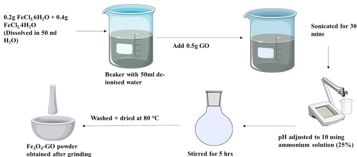
Figure S1: Schematic representation of synthesis protocol of Fe<sub>3</sub>O<sub>4</sub>-GO composite
