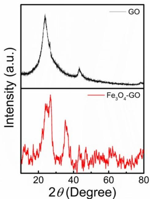
Figure S4: Powder XRD Spectrum of GO and Fe<sub>3</sub>O<sub>4</sub>-GO
