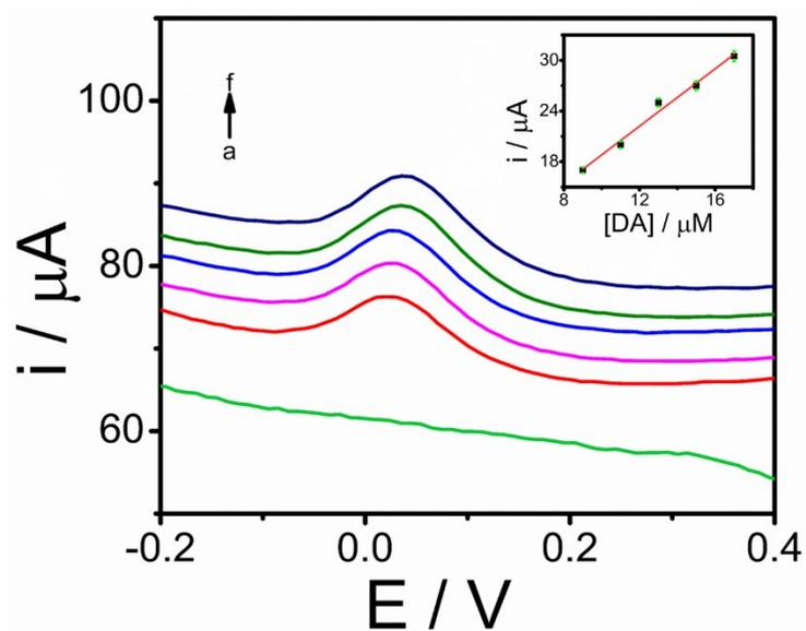
Figure S9: DPV responses of the microneedle sensor towards DA in the concentration range of 9  $\mu\text{M}$  to 17  $\mu\text{M}$  (in 0.1 M PBS) and linear plot between analyte concentration in  $\mu\text{M}$  (inset) and  $i / \mu\text{A}$  is provided in the inset.
