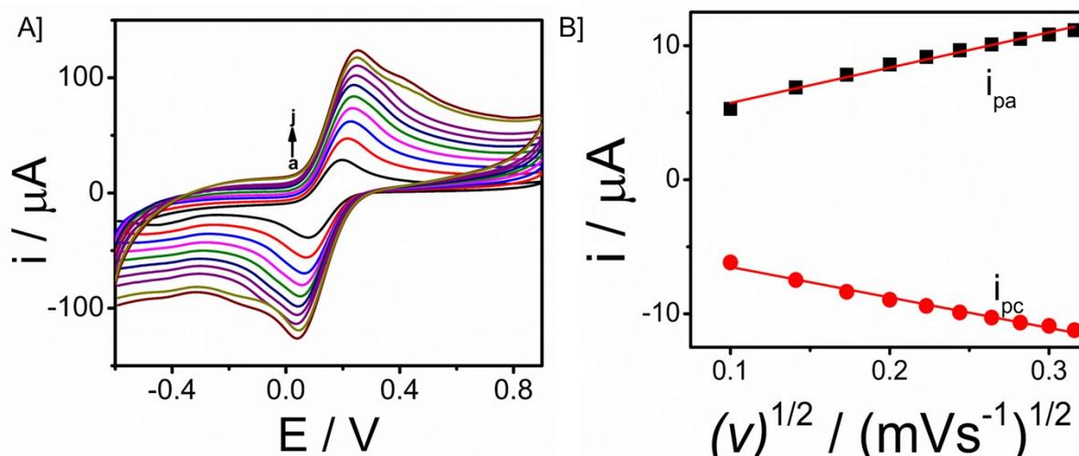
Figure S6: A] Effect of Scan Rate (10-100  $\text{mVs}^{-1}$ ) on Cyclic Voltammetry of CP/ $\text{Fe}_3\text{O}_4$ -GO/Chi in 10mM  $\text{K}_3[\text{Fe}(\text{CN})_6]$  + 0.1M KCl solution and.B] Plot of anodic ( $i_{pa}$ ) and cathodic peak ( $i_{pc}$ ) currents vs. scan rate.
