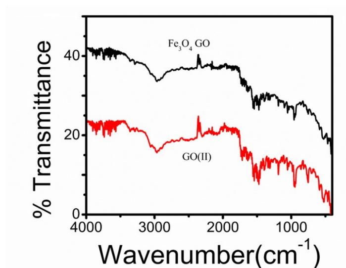
Figure S3: FTIR Spectrum of GO and Fe<sub>3</sub>O<sub>4</sub>-GO
