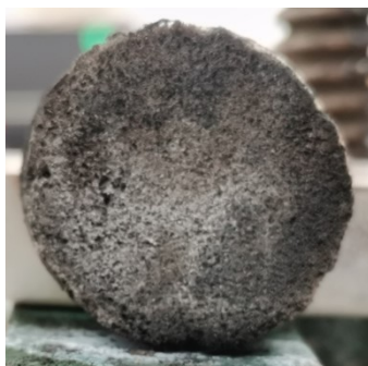
Fig. S17 Picture of the burning surface of the B-CSMC-X superfoam after being burned by a butane flame for 3600 s.
