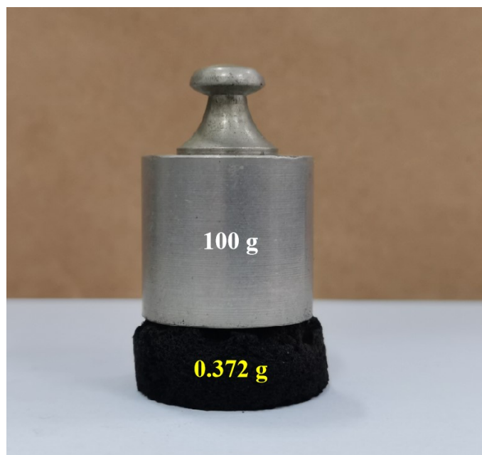
Fig. S12 The image of the B-CSMC-5.0 super foam could withstand about 269 times its own mass.
