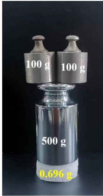
Fig. S9 The image of the CSMC-5.0 super foam could withstand 1005 times its own mass.
