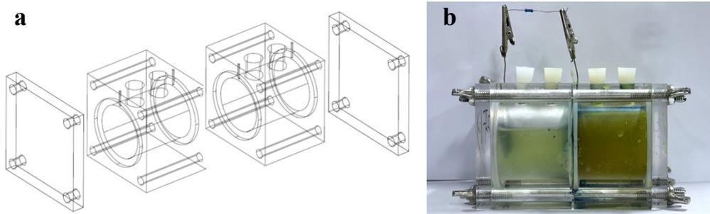
**Fig. S2** (a) MFC structure design sketch; (b) Physical drawing of MFC device.
