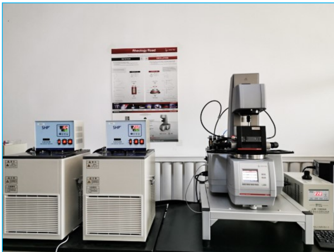
(a) MCR 702 dual drive modular rheometer
