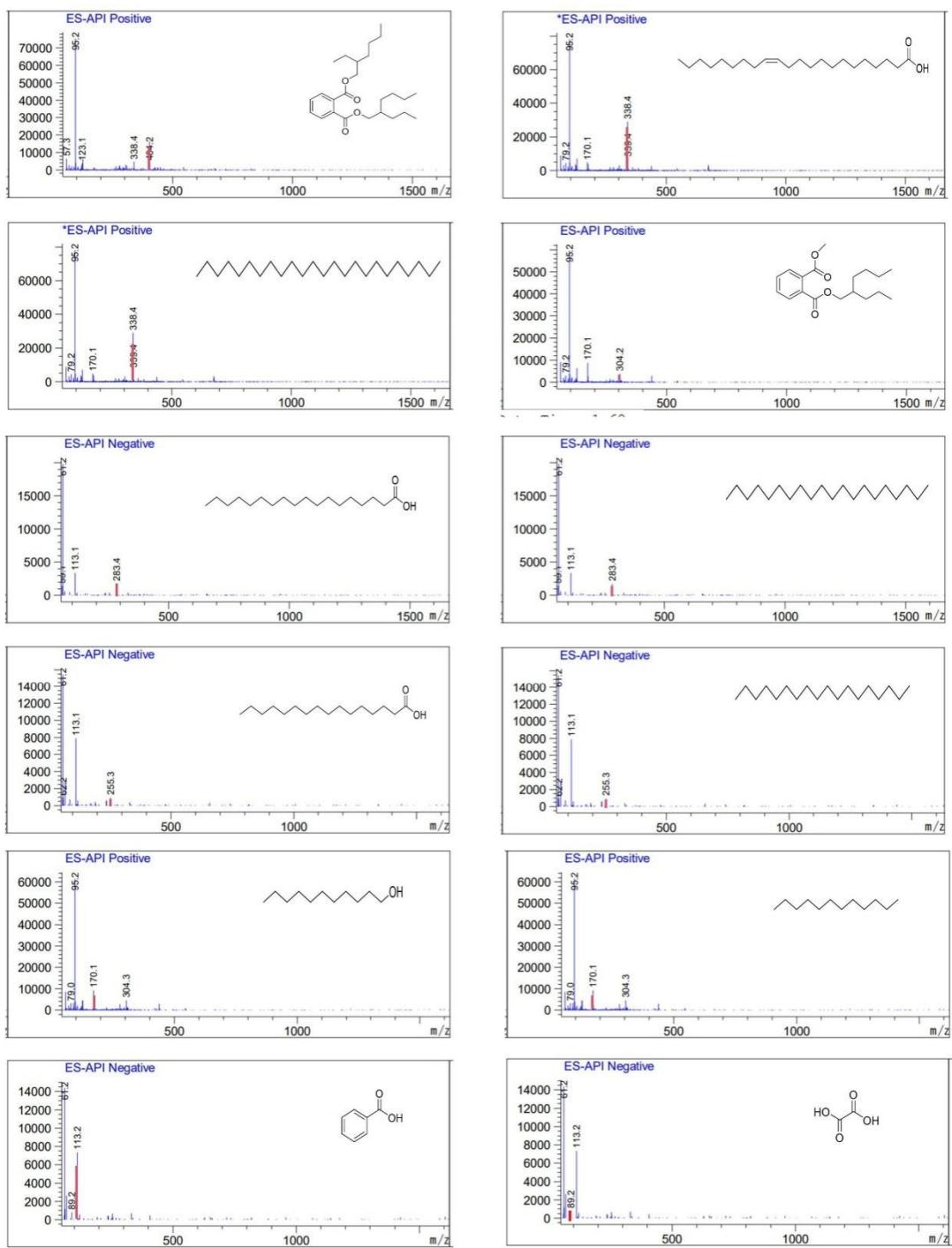
**Fig.S14.** The LC-MS spectra of degradation intermediates of PVC.
