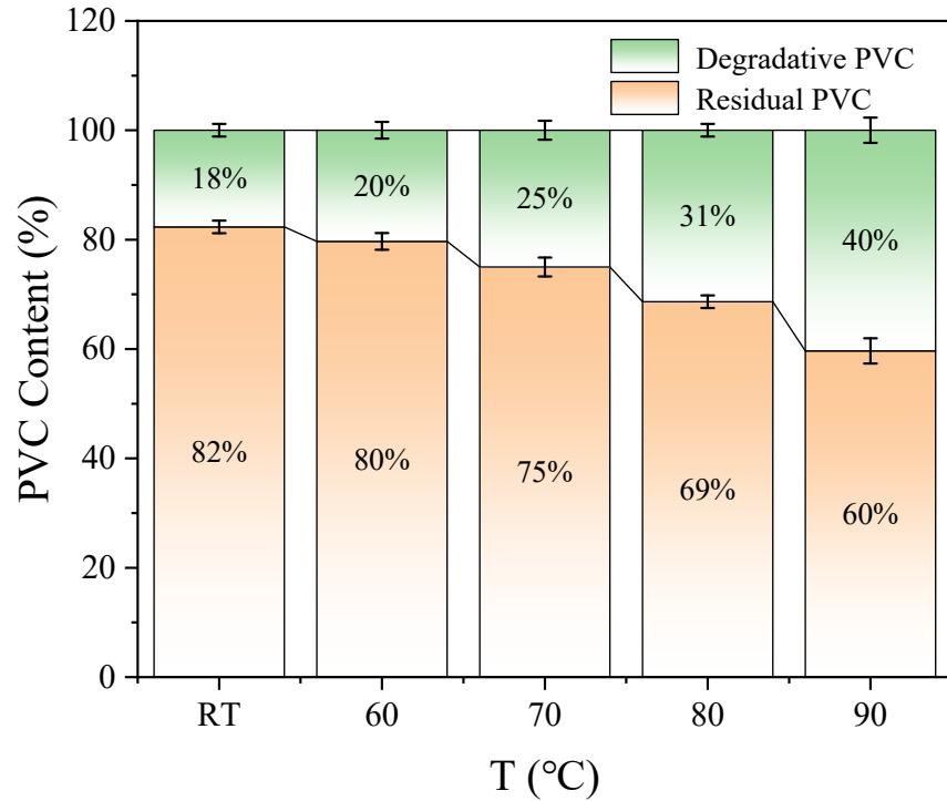
**Fig.S4.** Effect of temperature on degradation of PVC.
