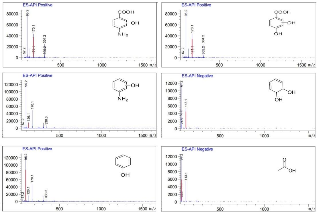
**Fig.S13.** The LC-MS spectra of degradation intermediates of PABA.
