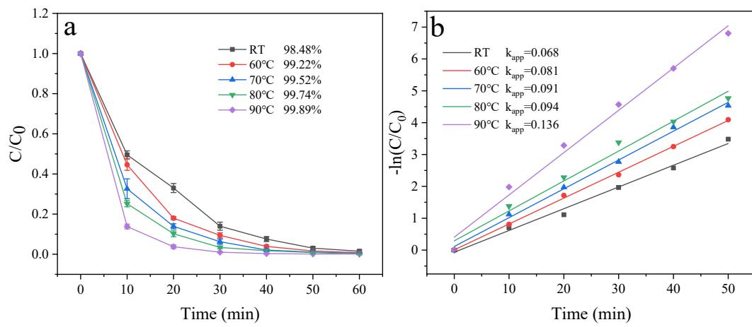
**Fig.S3.** (a) Effect of temperature on degradation of PABA. (b) First order kinetic line of degradation of PABA by temperature.
