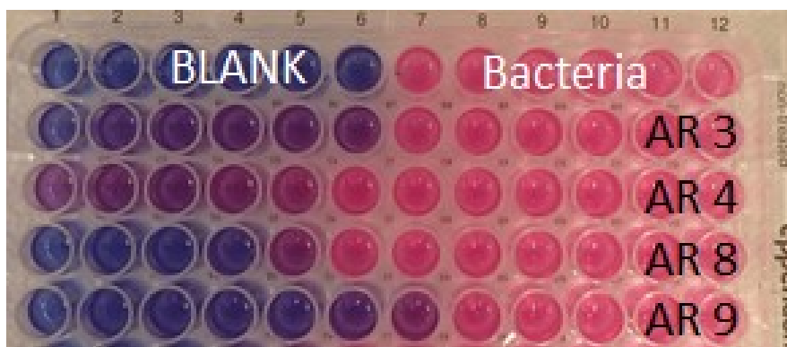
Figure S13: Culture media plates of Mycobacterium tuberculosis for the Anti- Mycobacterium tuberculosis activity of spiropyrrolidine heterocyclic hybrids (AR3-9 represent as compound 5c , 5d , 5h and 5i )
