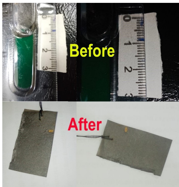
Fig. S7. Visible color change of PdCl 2 Strips: pre- and post-chemical reaction
