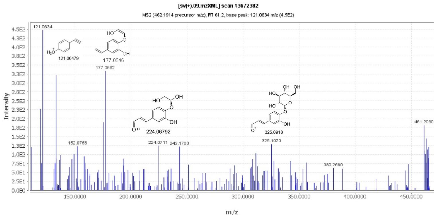
**Figure S13.** ESI-MS/MS spectrum of 4'''-*O*- $\beta$ -D-glucopyranosyl caffeoyltyramine (**1.27**).
