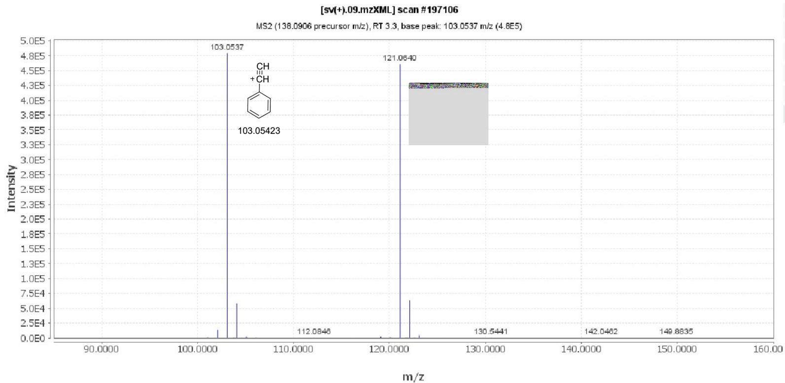
**Figure S5.** ESI-MS/MS spectrum of tyramine (1.6).
