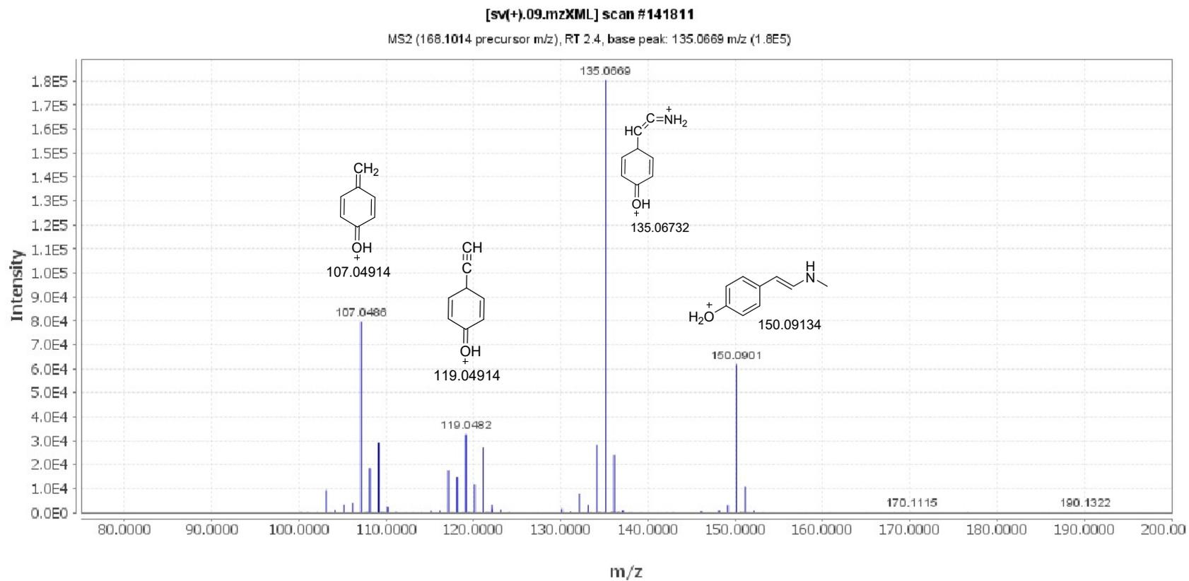
Figure S8. ESI-MS/MS spectrum of *N*-methyloctopamine (synephrine) (1.10).
