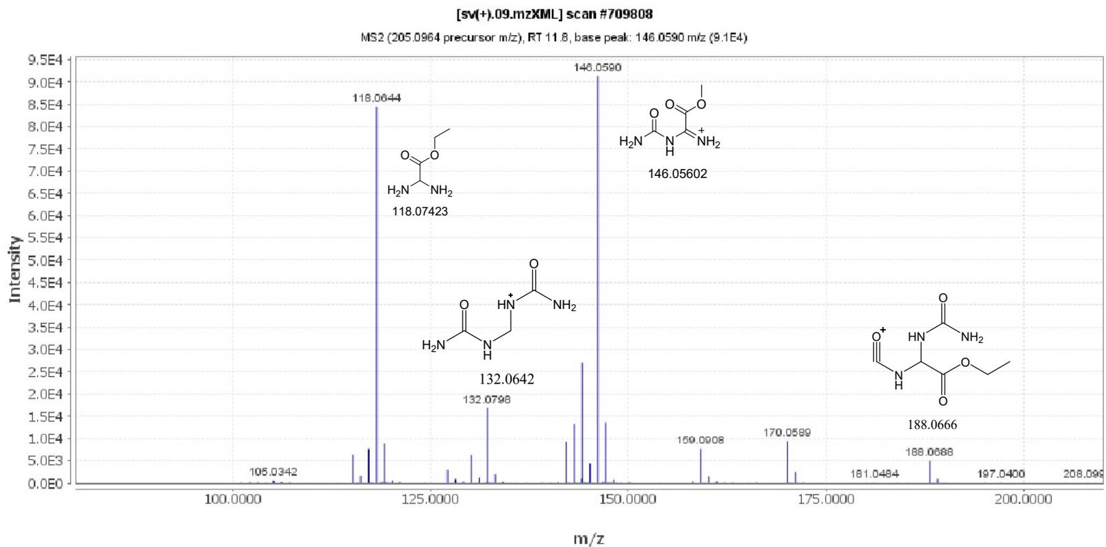
**Figure S15.** ESI-MS/MS spectrum of allantoic acid ethyl ester (**1.29**).
