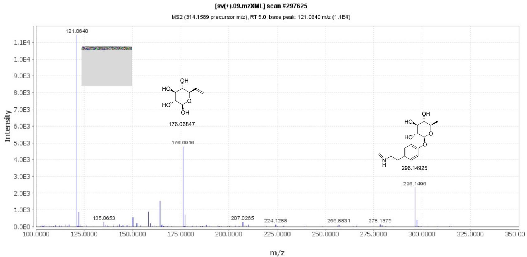
**Figure S10.** ESI-MS/MS spectrum of *N*-methyltyramine-*O*- $\beta$ -D-glucoside (**1.12**).
