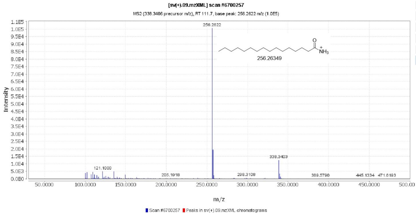
**Figure S18.** ESI-MS/MS spectrum of *N*-cyclohexanecarbonylpentadecylamine (**6.3**).
