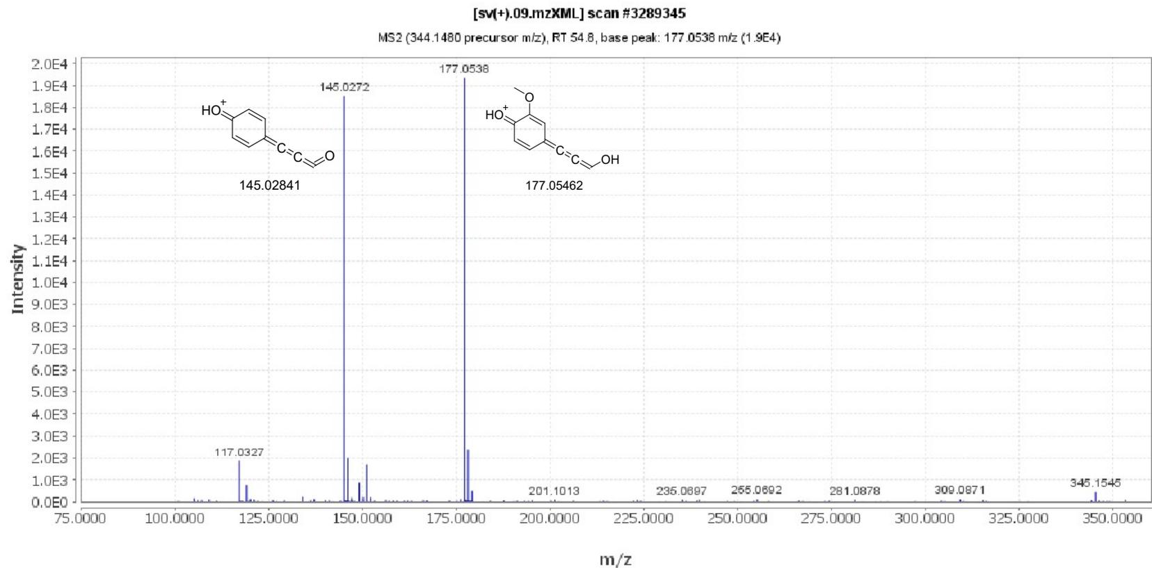
Figure S12. ESI-MS/MS spectrum of *N*-*trans*-feruloyl 3-*O*-methyldopamine (**1.25**).
