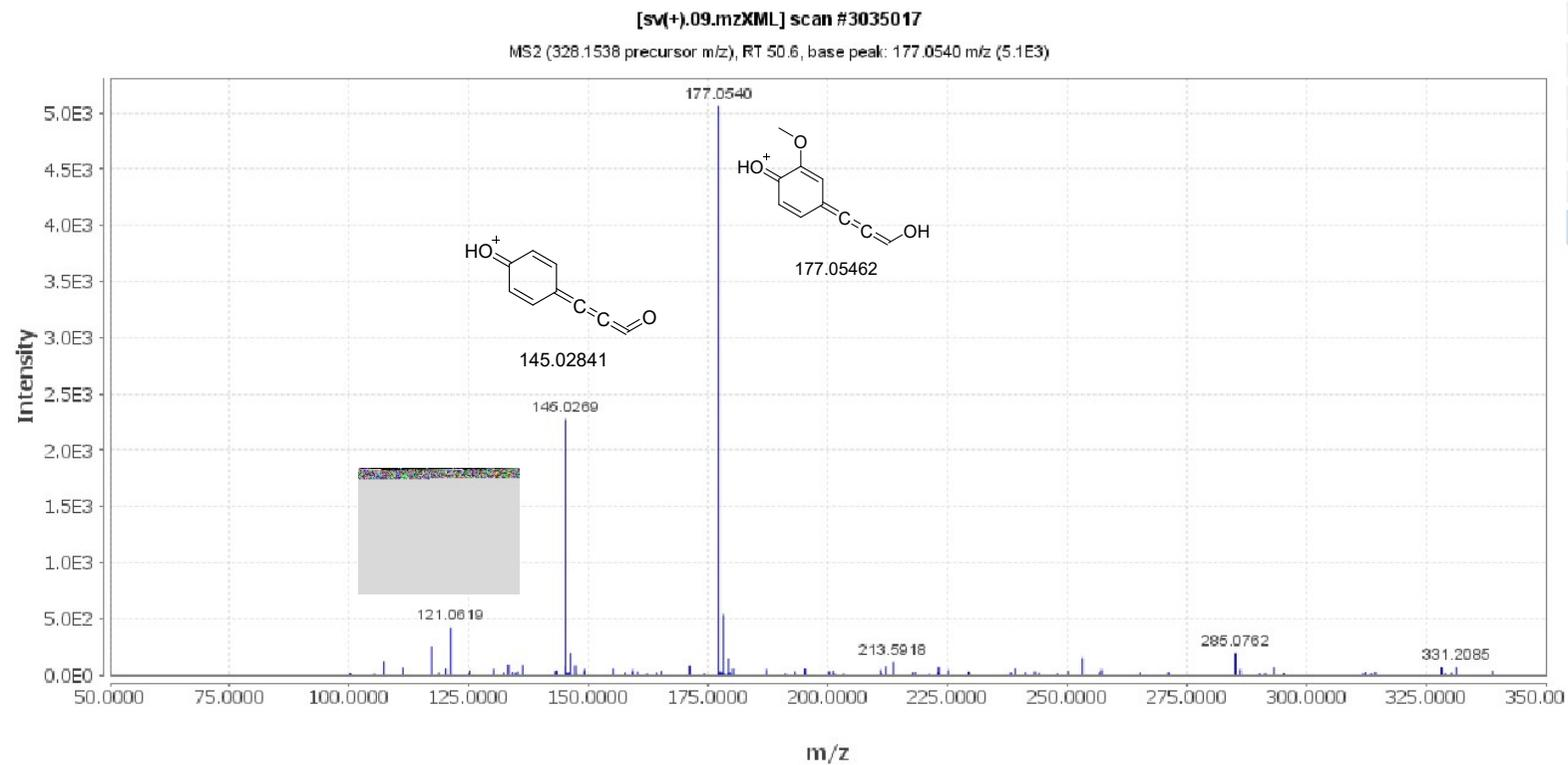
**Figure S11.** ESI-MS/MS spectrum of (*E*)-3-(4-hydroxy-3-methoxyphenyl)-*N*-(4-methoxyphenethyl)acrylamide (**1.23**).
