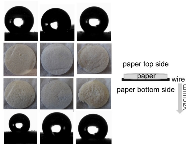
Figure S 4: Wettability of small papers made of fibres with a dense silica coating. The ‘close’ and ‘far’ side of the sieve show a hydrophobic character which indicates that the paper production process does not influence the wettability of the paper.
