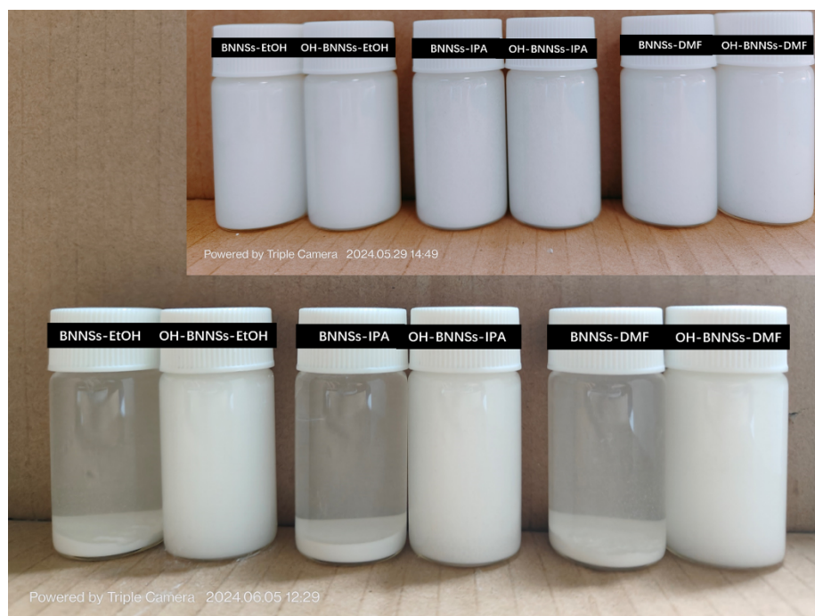
Fig. S7 Digital photograph images of BNNs and OH-BNNs suspensions in ethanol, IPA and DMF for 1 week after sonication. The inset shows digital photograph images of these three dispersions from a week ago.
