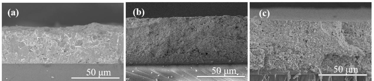
Figure S3 (a), (b), and (c) the complete Cross-sectional SEM images of perovskite about  $n=\infty$ ,  $n=10$ , and  $n=6$ , respectively
