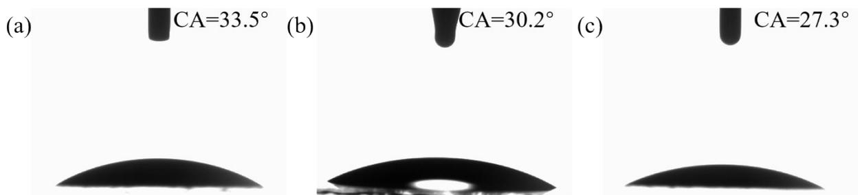
Figure S2 (a), (b), and (c) the contact angles of  $n=\infty$ ,  $n=10$ , and  $n=6$  perovskite precursor solutions on the substrate surface, respectively
