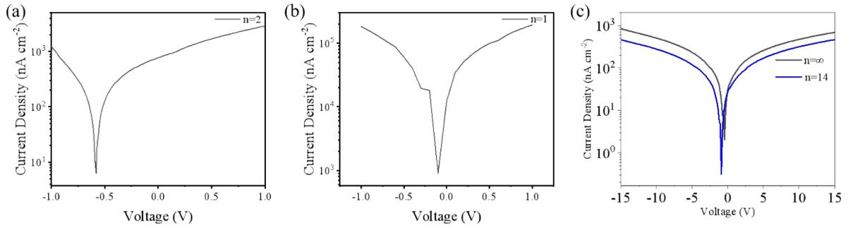
Figure S4 (a), (b) and (c) the J-V curve of  $n=2$ ,  $n=1$ , and  $n=14$  perovskite thick films, respectively
