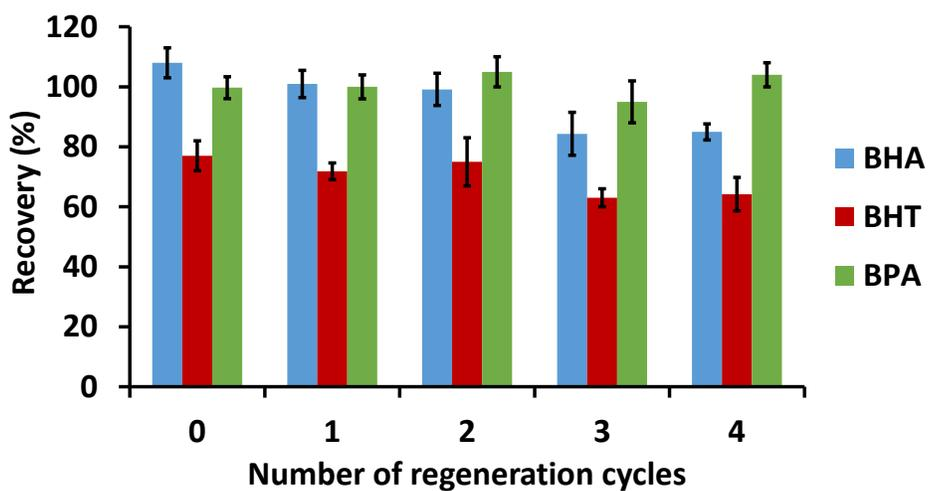
Fig. S6 Extraction recovery (%) of mC18/Pa/Alg during four regeneration cycles.
