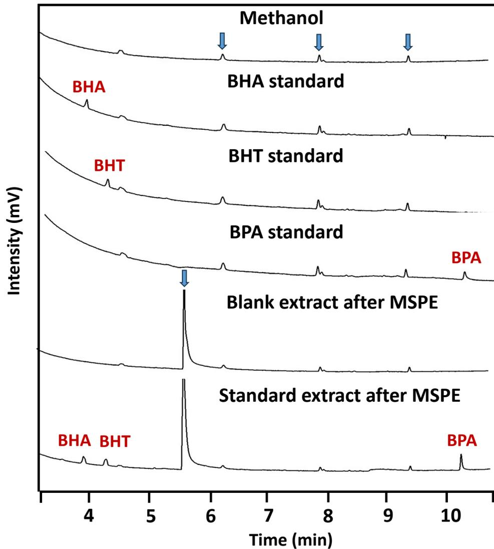
**Fig. S7** GC-FID chromatograms of methanol, a standard solution (single BHA, BHT and BPA), a treated blank extract after MSPE and a treated standard extract after MSPE.
