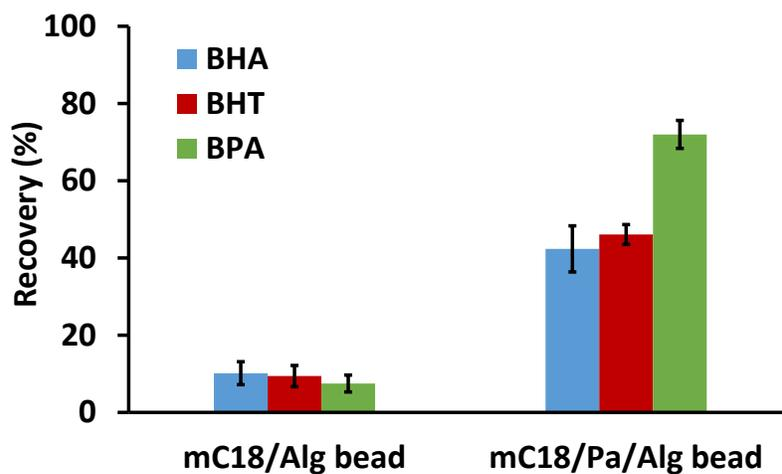
**Fig. S3** Comparison of the extraction efficiency of BHT, BHA and BPA between the mC18/Alg bead (without Pa) and the mC18/Pa/Alg bead (with Pa).
