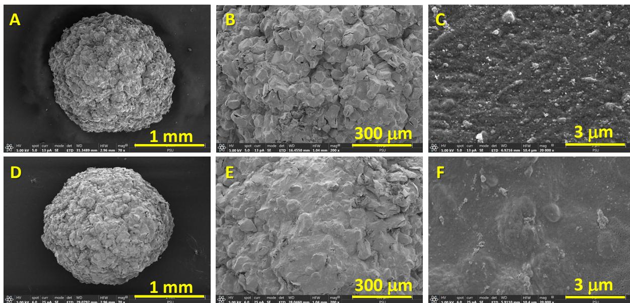
**Fig. S2** FE-SEM images show (A–C) the mC18/Pa/Alg bead (with Pa), and (D–F) the mC18/Alg bead (without Pa) at 70X, 200X, and 20,000X magnifications, respectively. Pa stands for paracetamol.
