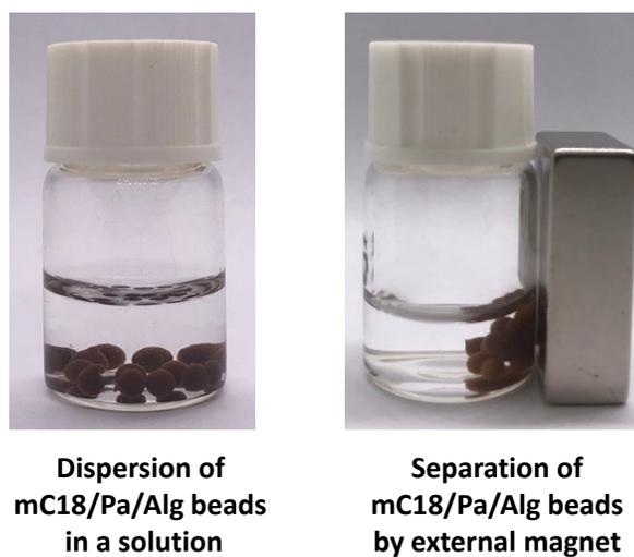
**Fig. S1** Dispersion and separation of the beads. The beads are easily separated from the water by an external magnet.
