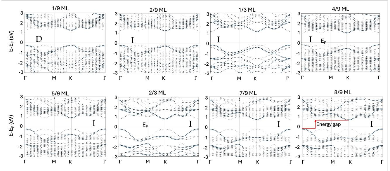
Figure 3: Effective band structures for different oxygen coverages in  $\text{MoSe}_2$ . Red arrow is to identify the band gap visually. D, and I stand for direct and indirect transitions, respectively.
