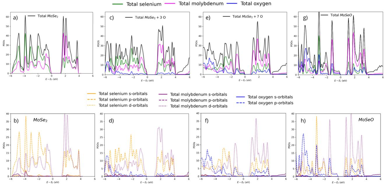
Figure 5: Projected density of states (PDOs) are separated per atom and per orbital. The labels a and b correspond to the pristine monolayer ( $MoSe_2$ ), b and c correspond to the monolayer with three oxygen atoms, e, and f correspond to the monolayer with seven oxygen atoms, and g and h correspond to the Janus monolayer  $MoSeO$ .
