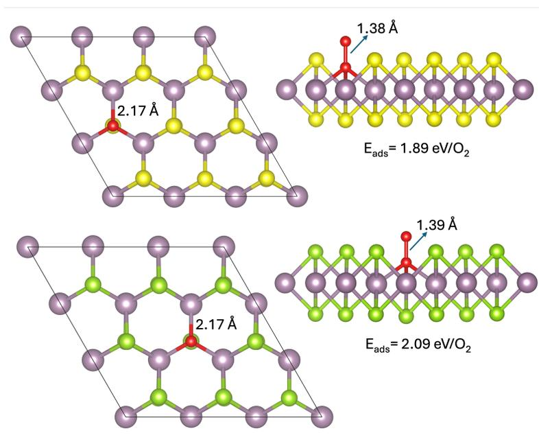
Figure 1: O<sub>2</sub> adsorption on the S/Se vacancy of MoS<sub>2</sub>/MoSe<sub>2</sub> monolayers.
