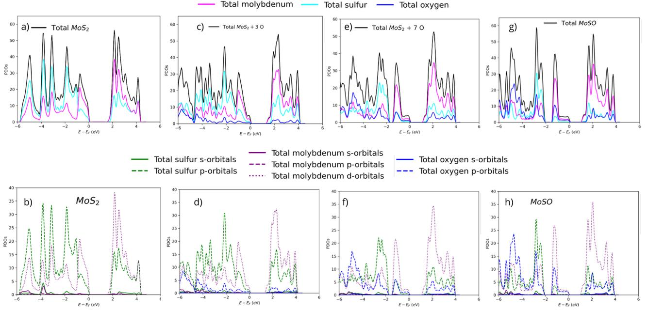
Figure 4: Projected density of states (PDOs) are separated per atom and per orbital. The labels a and b correspond to the pristine monolayer ( $MoS_2$ ), b and c correspond to the monolayer with three oxygen atoms, e and f correspond to the monolayer with seven oxygen atoms, and g and h correspond to the Janus monolayer  $MoSO$ .
