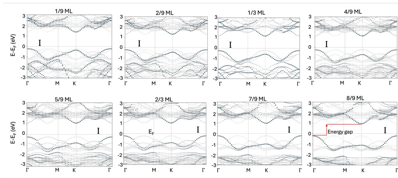
Figure 2: Effective band structures for different oxygen coverages in  $\text{MoS}_2$ . Red arrow is to identify the band gap visually. I stands for indirect transition.
