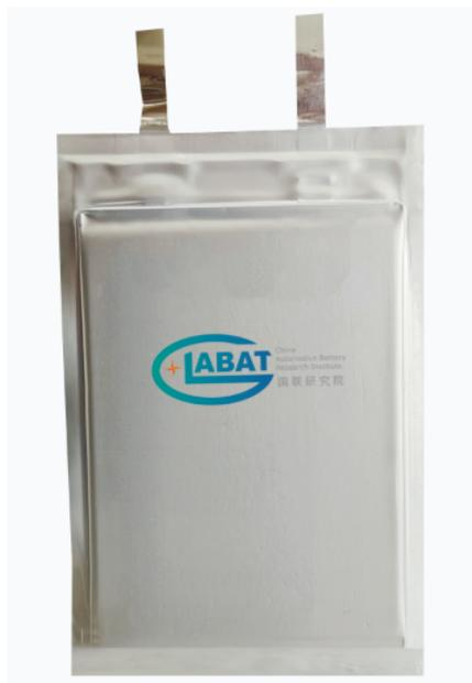
**Fig. The photo of the pouch cell prepared for research**
