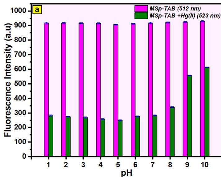
**Fig. S2a.** The changes in the fluorescence intensity at the range 512-523 nm of *MSp-TAB* and *MSp-TAB* + Hg(II) (0.15 g/L EtOH/H<sub>2</sub>O; 30/70, each; response time: 120 min, temperature: 25 °C) suspension mixtures at different pH (1.0-10.0).
