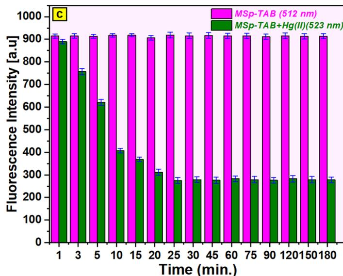
**Fig. S2c.** The changes in the fluorescence intensity at the range 512-523 nm of *MSp-TAB* and *MSp-TAB* + Hg(II) to determine response times. (Experimental conditions: 0.15 g/L EtOH/H<sub>2</sub>O; 30/70, each, pH: 7.0, and temperature: 25 °C).
