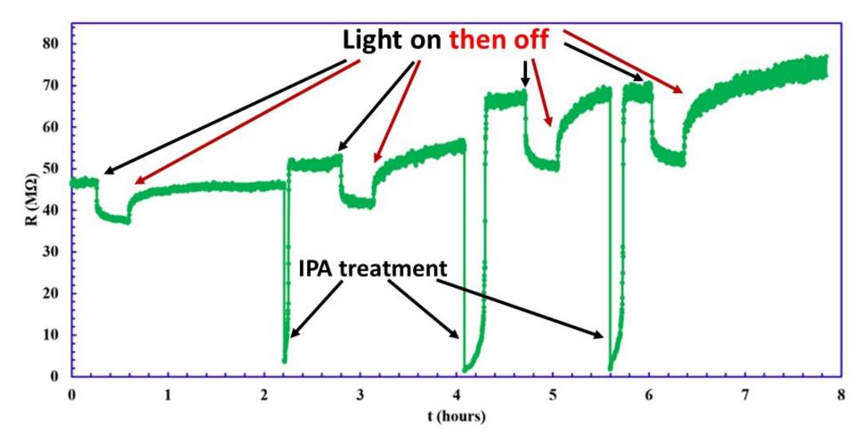
ZnO:Sb wire resistance versus time. IPA treatment causes the resistance to rise. Yet, turning the light on causes a larger drop in resistance compared to the untreated sample. So, the IPA treatment makes the sample surface more sensitive to light treatment.
