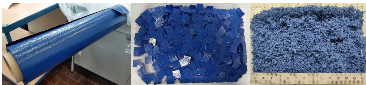
Figure S2 Photos of the PVC sample (left) as receive; (middle) cut in 1x1 cm flakes; (right) cryogenically milled to <4 mm.
