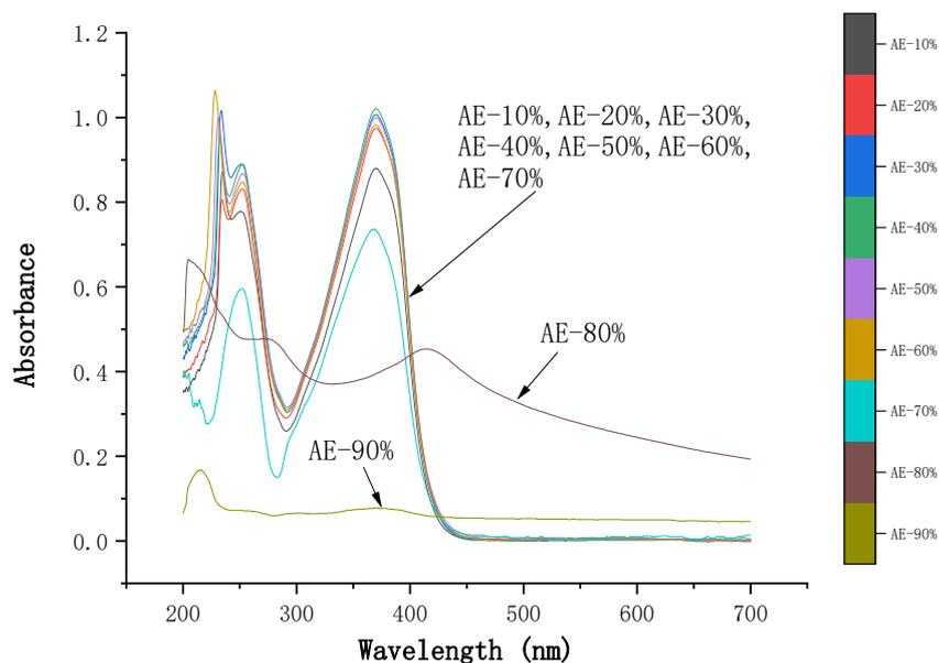
Figure S 3 the UV spectra of AE-3 (10 μM) in a THF/phosphate buffer (50 mM, pH=7.4) with different water content.
