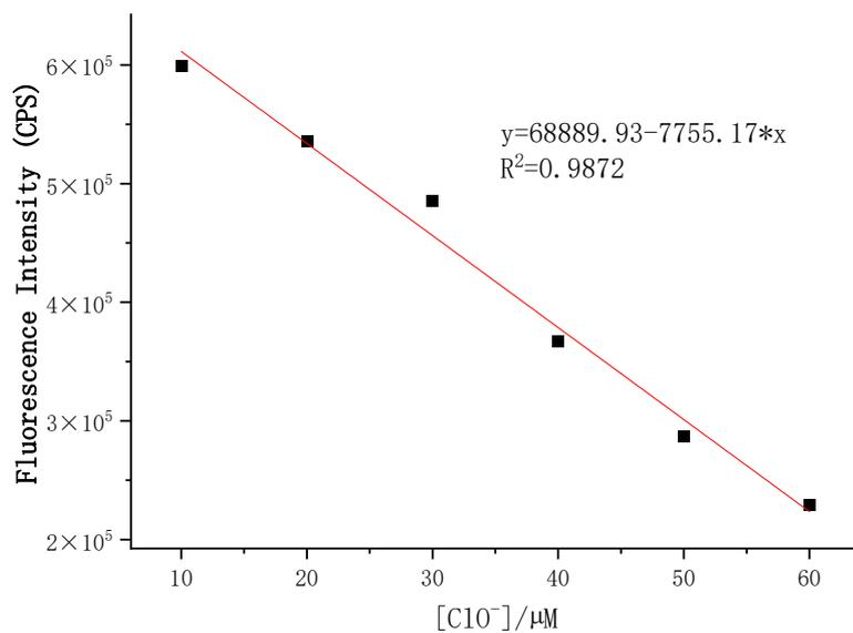
Figure S 11 The linear relationship between fluorescence intensity at 556nm of AE-3 (10 μM) and HClO
