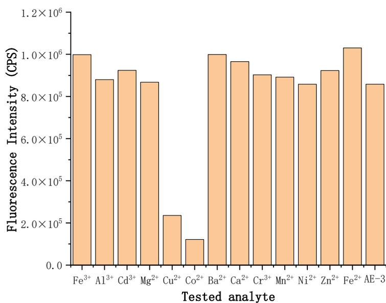
Figure S 4 The 556nm fluorescence intensity of the AE-3 (10 μM) in the presence of different analytes (10
