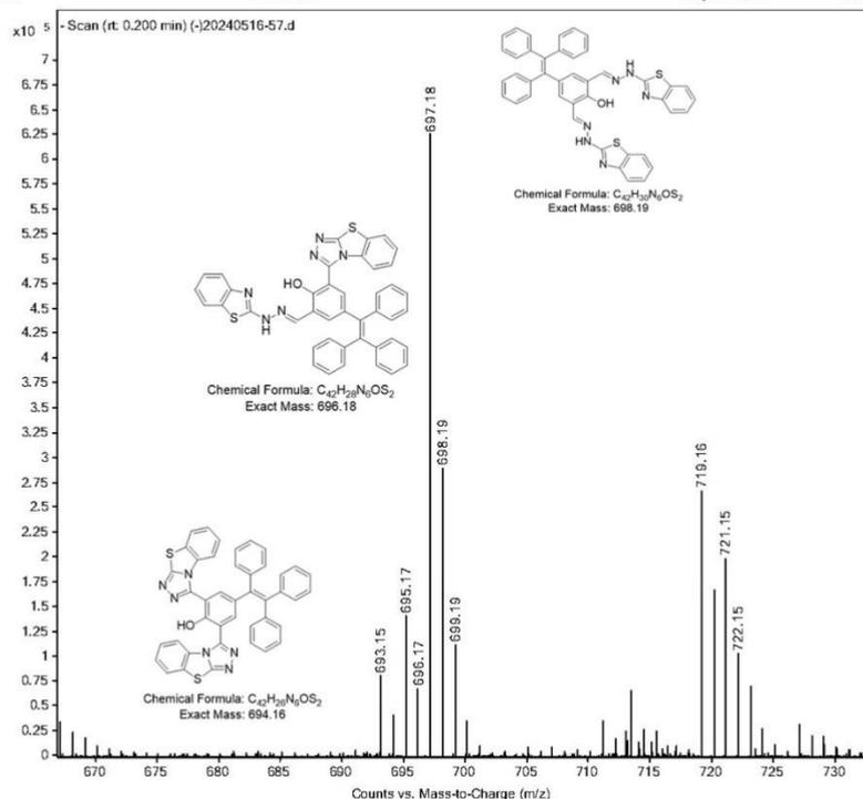
Figure S 21 The mass spectrum following the reaction of compound AE-3 with hydrazine.
