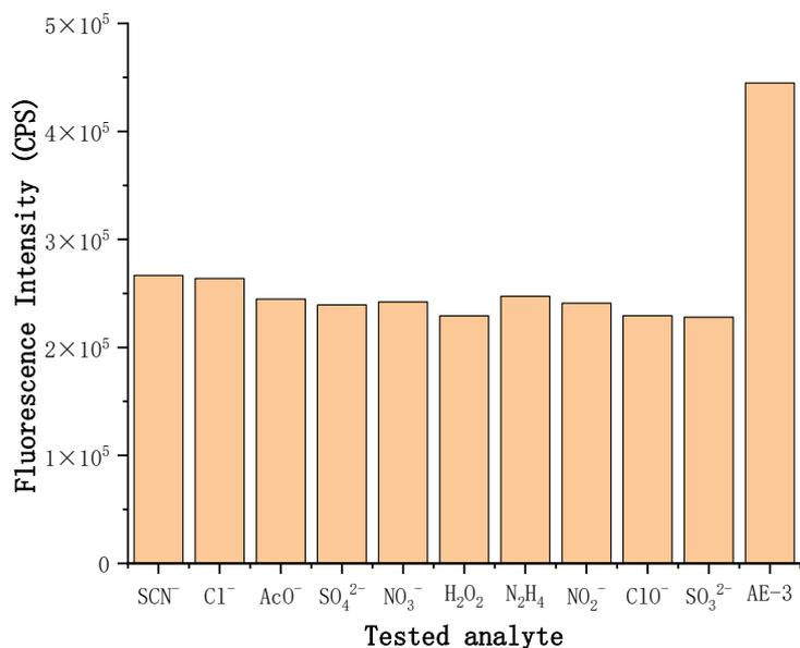
Figure S 9 The fluorescence intensity at 556nm bar graph of the AE-3 (10  $\mu\text{M}$ ) and HClO (50  $\mu\text{M}$ ) in the presence of different analytes (50  $\mu\text{M}$ ) in THF/phosphate buffer (1/9, v/v, 50 mM, pH=7.4)
