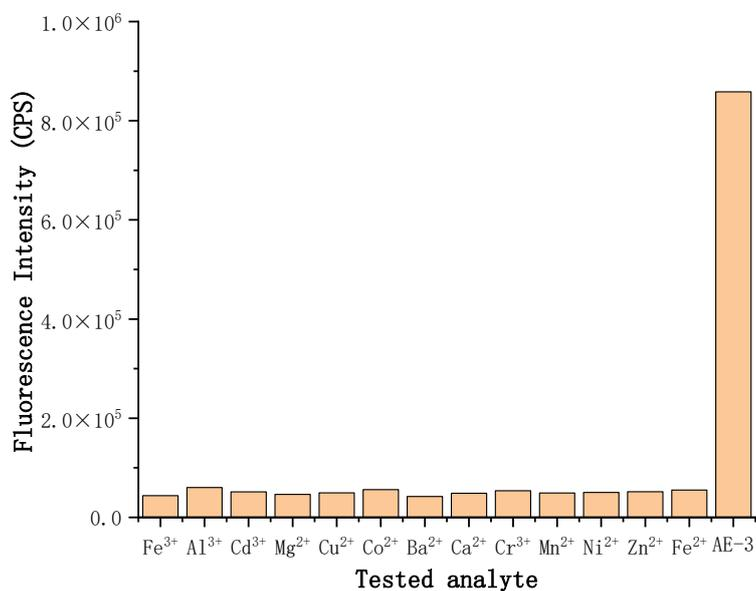
Figure S 5 The 556nm fluorescence intensity of the AE-3 (10  $\mu\text{M}$ ) and Co<sup>2+</sup> (10  $\mu\text{M}$ ) in the presence of different analytes (10  $\mu\text{M}$ ) in THF/phosphate buffer (1/9, v/v, 50 mM, pH=7.4).
