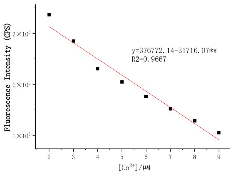
Figure S 6 The linear relationship between 556nm fluorescence intensity of AE-3 (10  $\mu\text{M}$ ) and Co<sup>2+</sup> (0.1-0.9  $\mu\text{eq}$ ).
