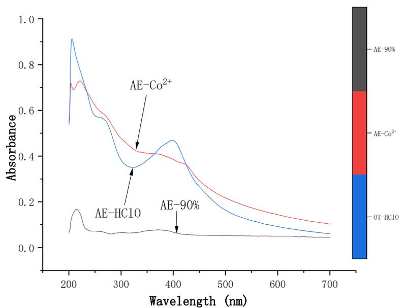
Figure S 12 UV spectra of the probe alone, with hypochlorous acid, and with cobalt ions in THF/phosphate buffer ( 50 mM, pH=7.4).
