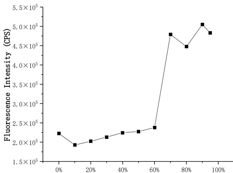
Figure S 1 The relationship between the fluorescence intensity of AE-3 (10  $\mu$ M) at 556nm and different water content (0%-99%) in THF/phosphate buffer ( 50 mM, pH=7.4)
