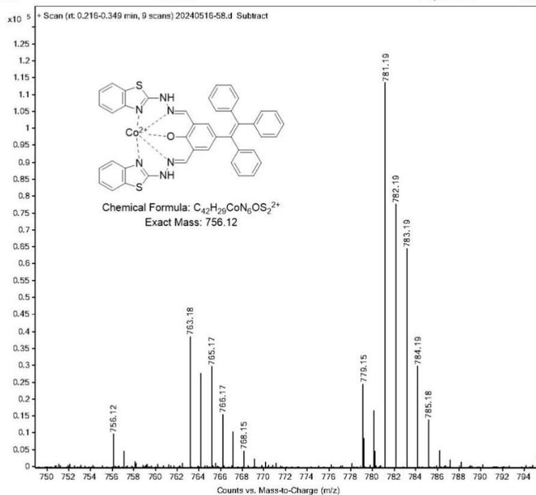
Figure S 20 The mass spectrum of compound AE-3 after chelation with cobalt ions
