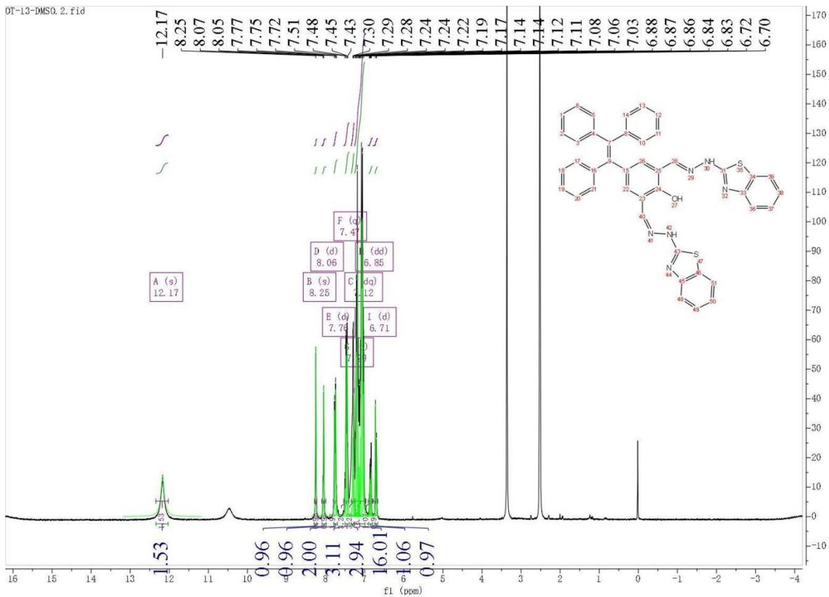
Figure S 15 The NMR Hydrogen Spectrum of AE-3
