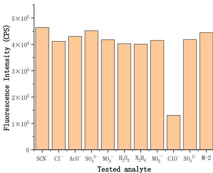
Figure S 8 The fluorescence intensity at 556nm bar graph of the AE-3 (10  $\mu$ M) in the presence of different analytes (50  $\mu$ M) in THF/phosphate buffer (1/9, v/v, 50 mM, pH=7.4)
