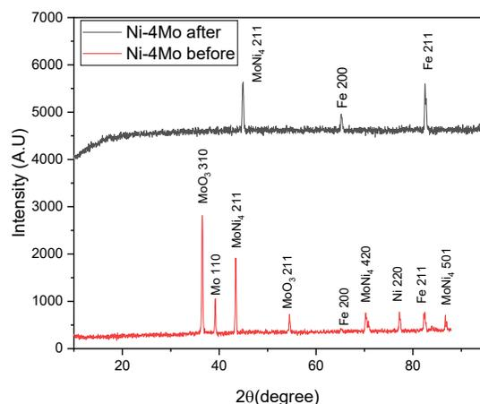
Fig. S4: XRD of Ni-4Mo catalyst before and after stability test.
