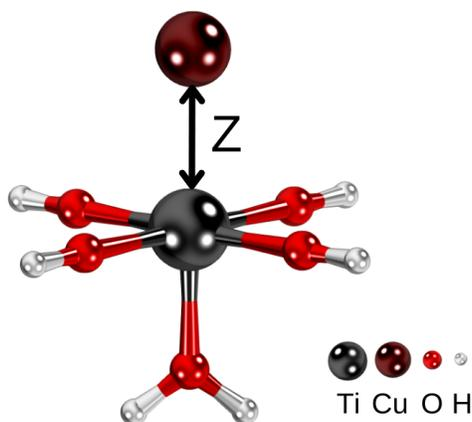
Fig. S2 Cu-TiO<sub>5</sub>H<sub>6</sub> complex used for benchmark study. Z is defined as the distance between the Cu and Ti atoms.
