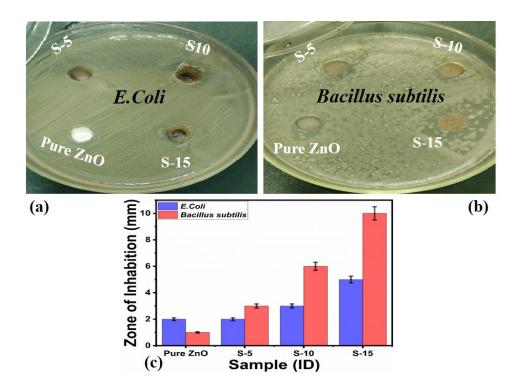
**Figure (S2):** (a, b) Antibacterial activity of pure ZnO and ZnO nanostructures synthesized with 5mL (S-5), 10mL(S-10) and 15 mL(S-15) of Moringa *oleifera* leaves extract respectively in E.Coli and their petri dish view with inhibition zone, (c) Corresponding measured inhibition zone in mm.
