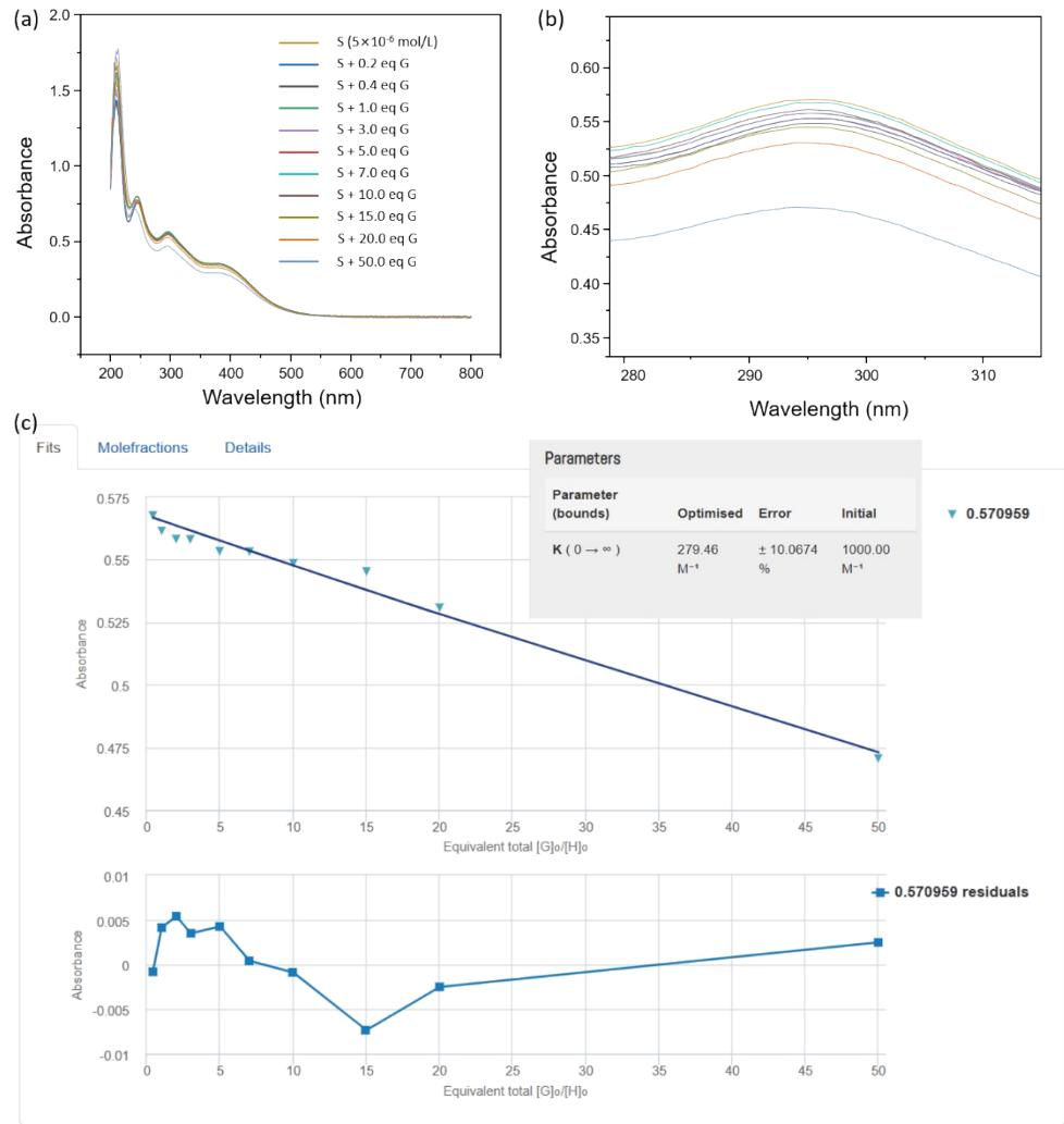
**Figure S26.** (a) The UV-vis spectra of GCS titration experiment. (b) The zoom in UV-Vis spectra of GCS titration experiments at 280 nm-310 nm. (c) The calculation of quantitative binding constants for GCS.
