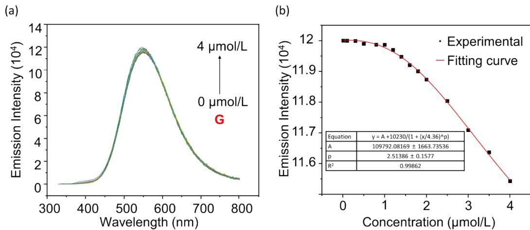
**Figure S24.** (a)The fluorescence spectrum of **GCS** which concentration was 0–4  $\mu\text{mol/L}$ . (b)The measured (dot) emission peak intensities and their corresponding linear test (solid lines).
