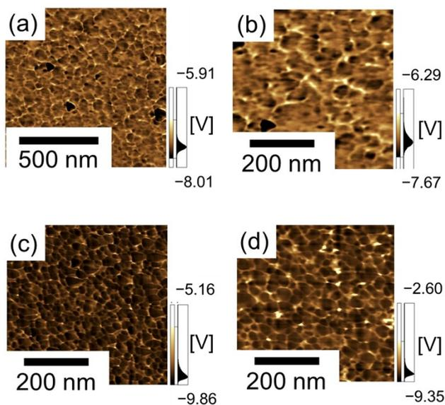
**Figure S4.** AFM phase images of the precipitated surfaces on (a) Mg, (b) Mg-KH<sub>2</sub>PO<sub>4</sub>, (c) Mg-K<sub>2</sub>HPO<sub>4</sub> and (d) Mg-K<sub>3</sub>PO<sub>4</sub> after the immersion into 1.5SBF.
