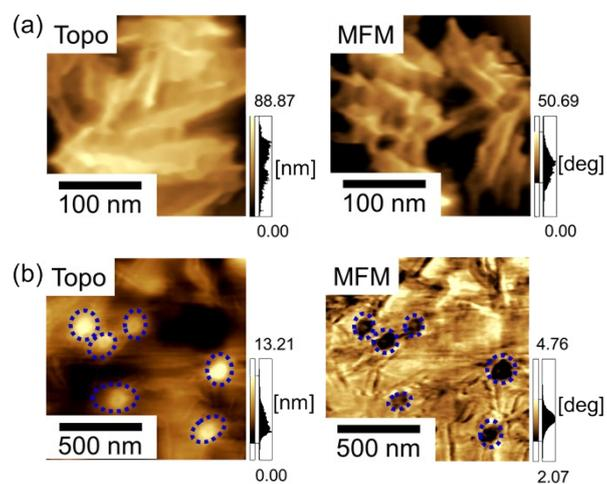
**Figure S1.** AFM topographic and MFM images of EPD films on the QCM-D gold sensor surfaces of (a) HA nanocrystals and (b) HA nanocrystal-precipitated Mgn NPs. The blue-colored dotted circles indicated the Mgn NPs shapes.
