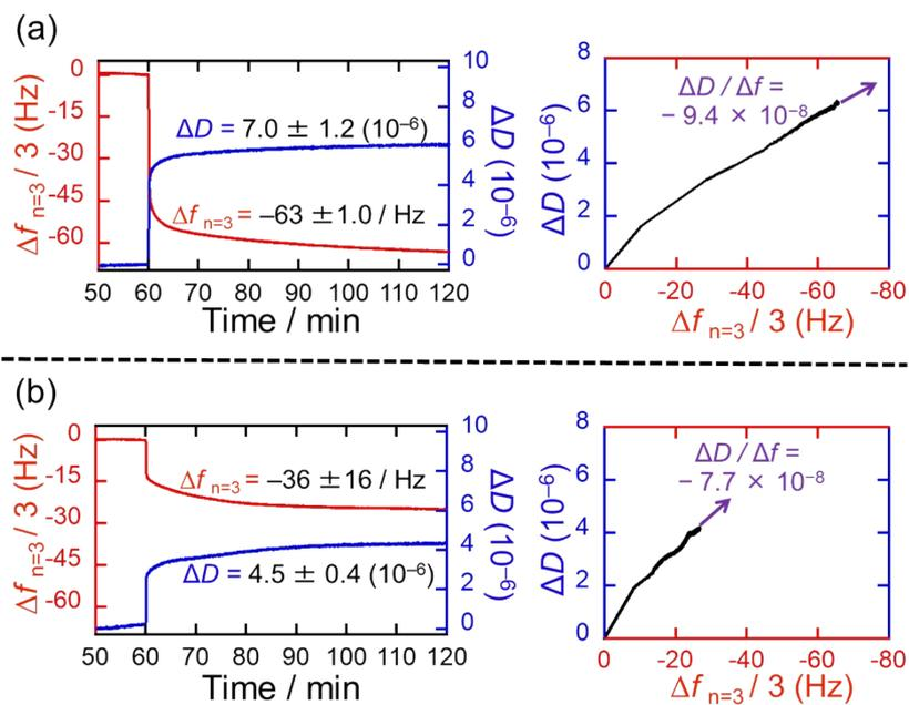
**Figure S3.**  $\Delta D$  and  $\Delta f$  curves and  $\Delta D$ - $\Delta f$  plots with the adsorption processes (a) 10 vol%FBS/PBS and (b) 10 vol%FBS/ $\alpha$ MEM on Mgn thin film.
