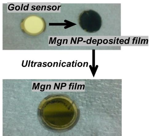
**Figure S2.** Photographs of the QCM-D gold sensor surfaces before and after the EPD of the MgNPs from the dispersion liquid at the solid weight of 0.8 wt%, and the MgNP film surface with the subsequent ultrasonication treatment at the thickness measured by QCM of  $71 \pm 36$  nm (density of Mg:  $5.2 \text{ g} \cdot \text{cm}^{-3}$ ).
