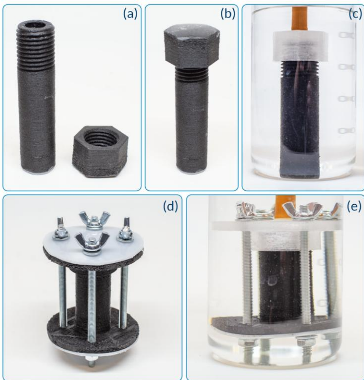
Figure S14. Impermeability tests inside alcohol media for I-tube type 3 (a-c) and I-tube type 4 reactors made of PP-GF30 (d, e).
