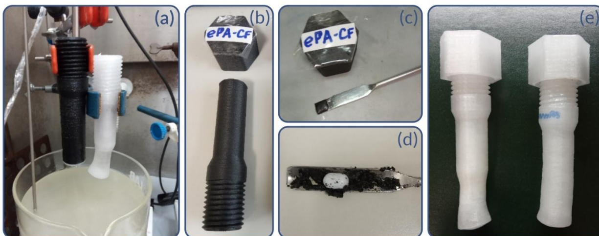
Figure S23. Plastic reactors after heating experiments: (a) PP-GF30 and PETG; (b) PA-CF; (c), (d) deformation of the inner surface of the PA-CF reactor; (e) PETG reactors after the heating experiment - exposure to chemical (left) and thermal (100 °C, right) factors
