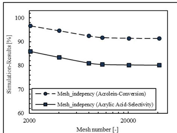
**Figure 5:** Effect of mesh numbers on calculated acrolein conversion and acrylic acid selectivity by CFD model for the case of the PBR (at 1 bar, 613 K, GHSV of 2000 h<sup>-1</sup>, and Oxygen/Acrolein ratio of 2).
