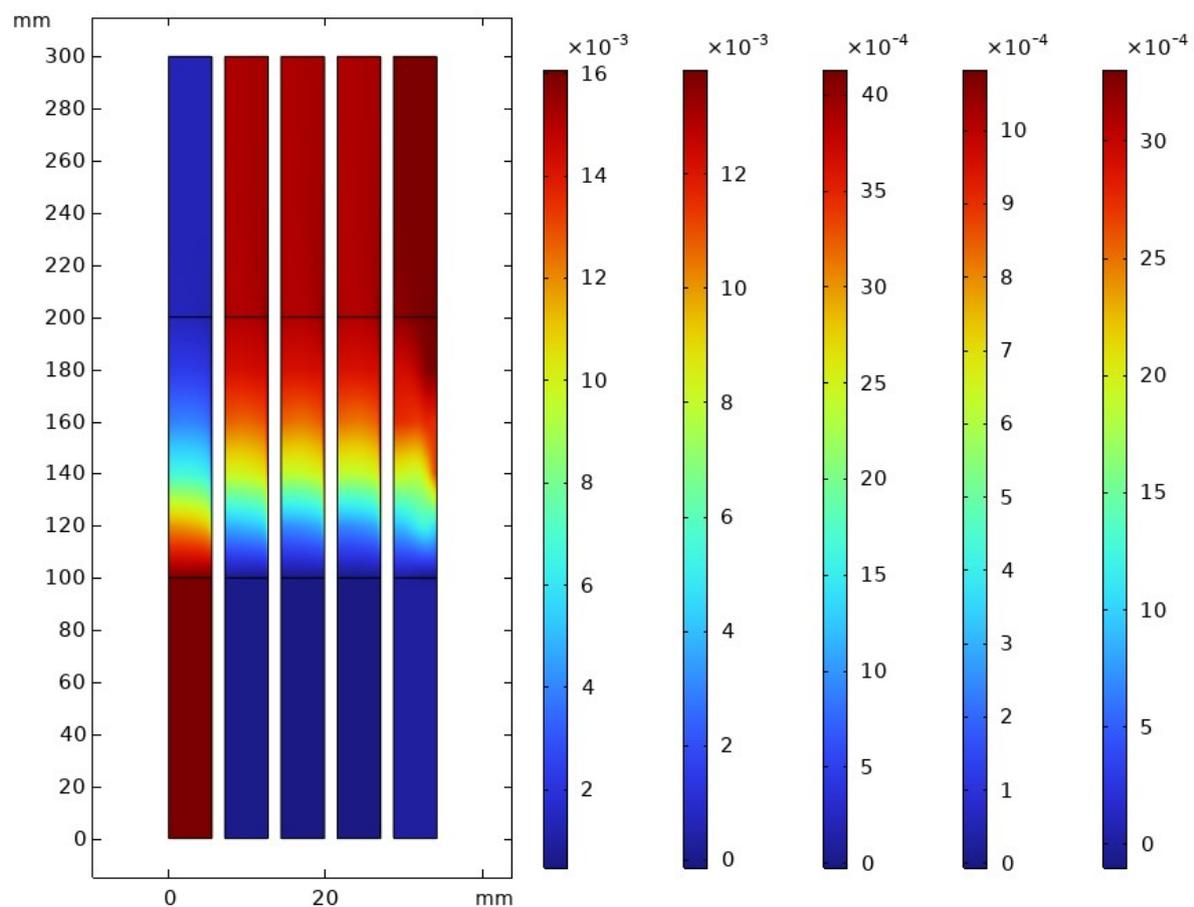
**Figure 8:** Concentration contours achieved by CFD simulation during acrolein oxidation in the PBR (acrolein, acrylic acid, carbon dioxide, carbon monoxide, and steam in order from left to right)
