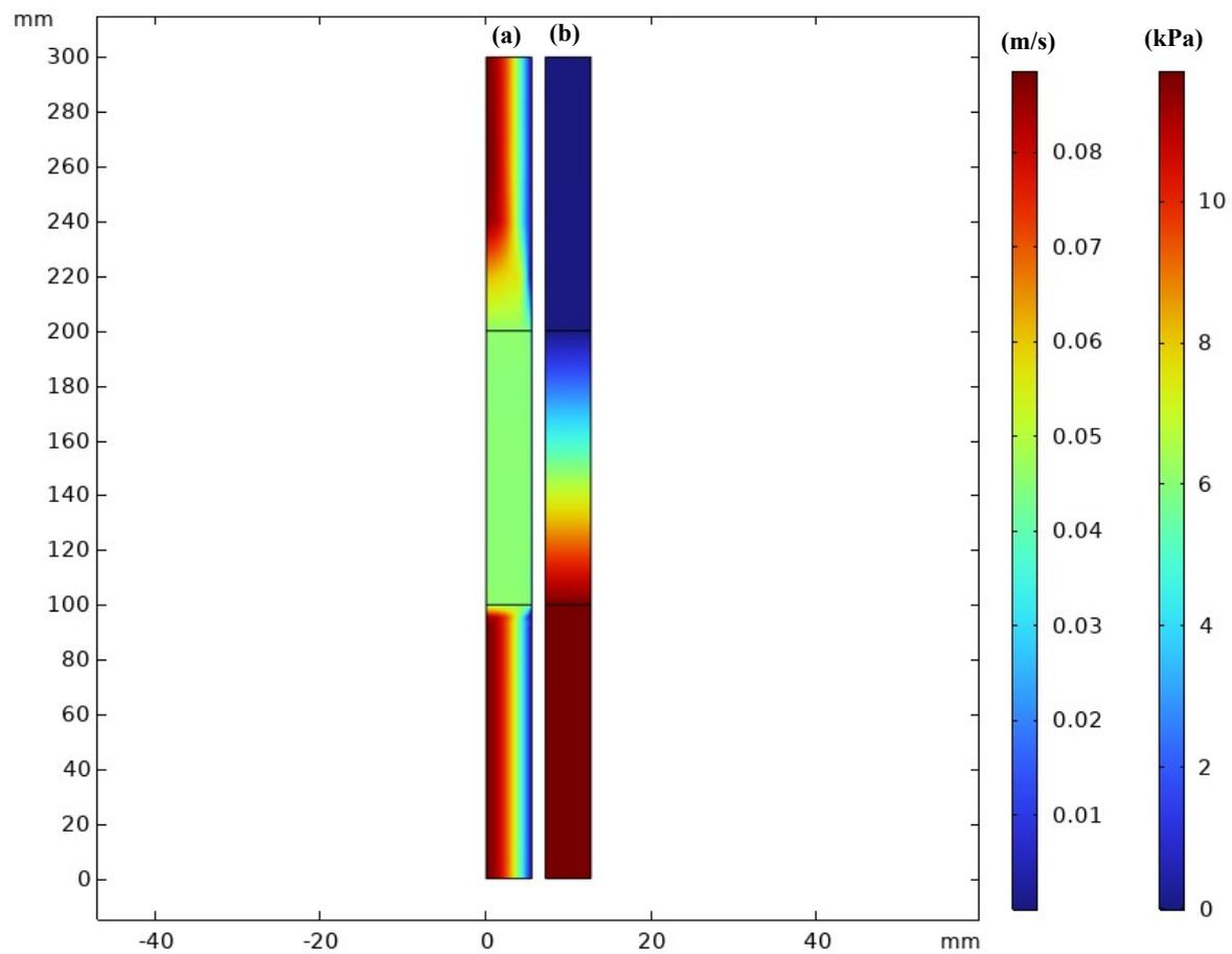
**Figure 9:** (a) Velocity contour (m/s), (b) Pressure contour (kPa) during acrolein oxidation in the PBR.
