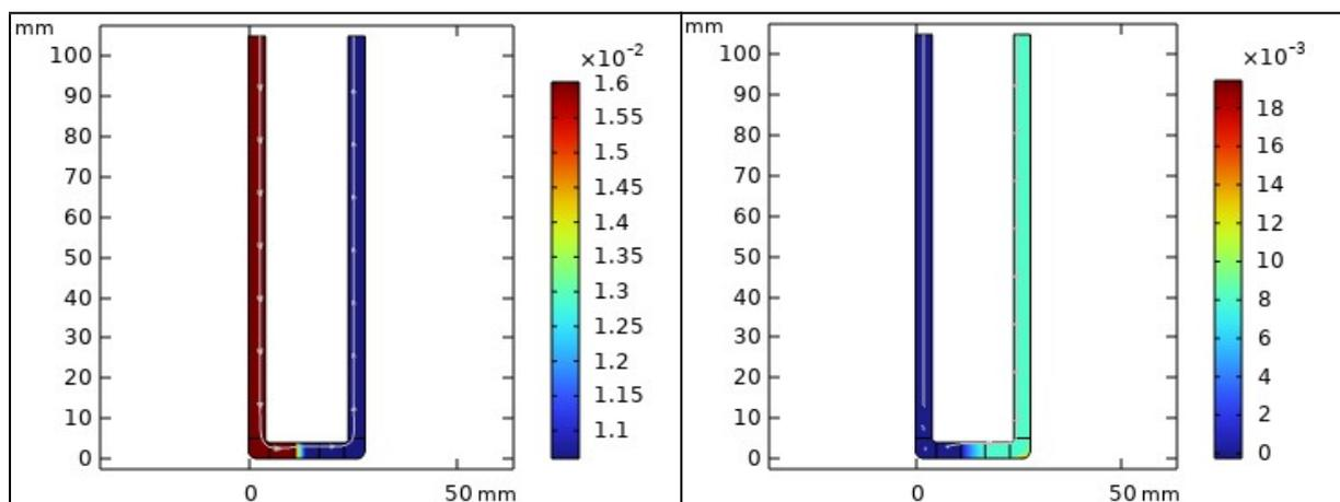
**Figure 7:** (a) Acrolein concentration distribution and (b) Acrylic acid concentration distribution in experimental setup presented by literature.
