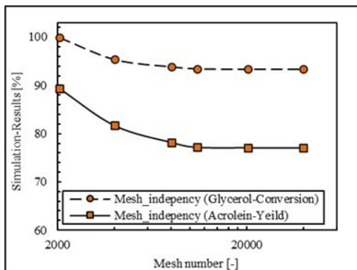
**Figure 1:** Effect of mesh numbers on calculated glycerol conversion and acrolein yield by CFD model for the case of the PBR (at a reaction pressure of 1 bar, reaction temperature of 613 K, GHSV of 4000 hr<sup>-1</sup> and glycerol mass fraction of 0.1).
