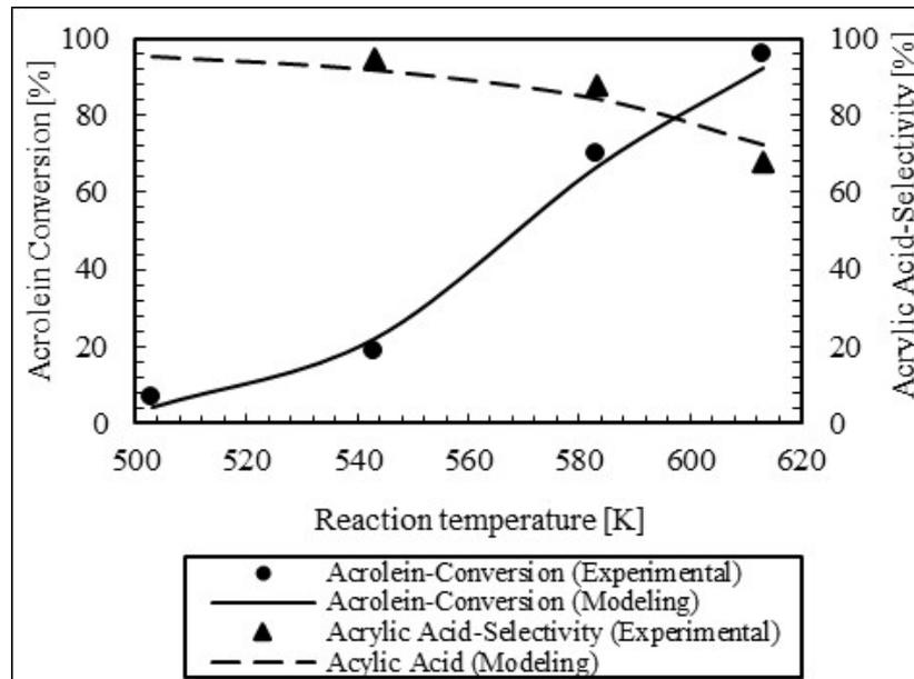
**Figure 6:** Comparison of the presented CFD results with experimental data provided by literature.
