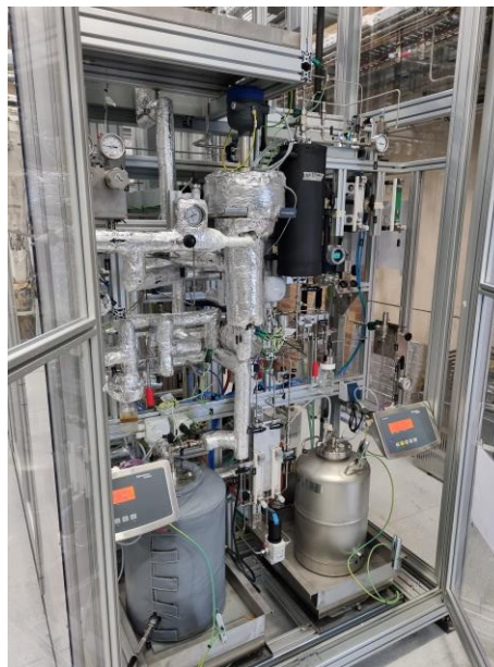
The hot separator (insulated) and cold separator (insulated black)
