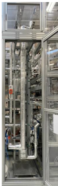
The (insulated) FT reactor tube
