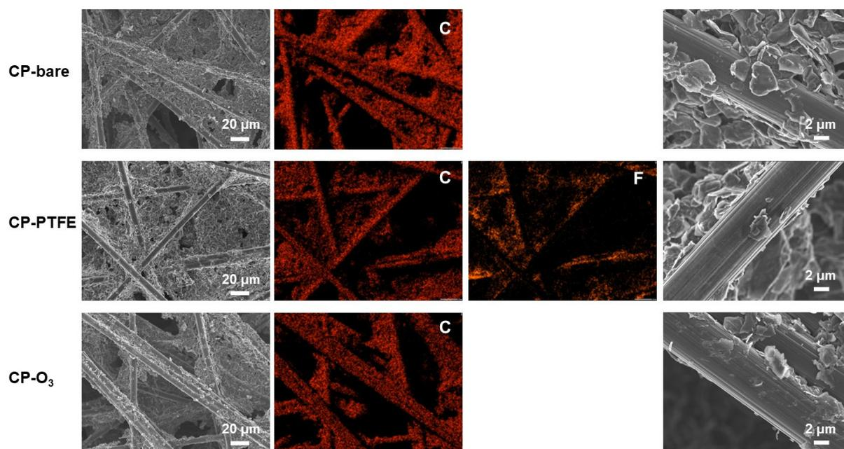
**Figure S2.** Scanning electron microscope (SEM) images of the surfaces of carbon paper (CP-bare), carbon paper loaded with PTFE (CP-PTFE), and ozone-treated carbon paper (CP-O<sub>3</sub>). Energy dispersive X-ray spectroscopy (EDS) mapping of carbon and fluorine for CP-bare and CP-PTFE.
