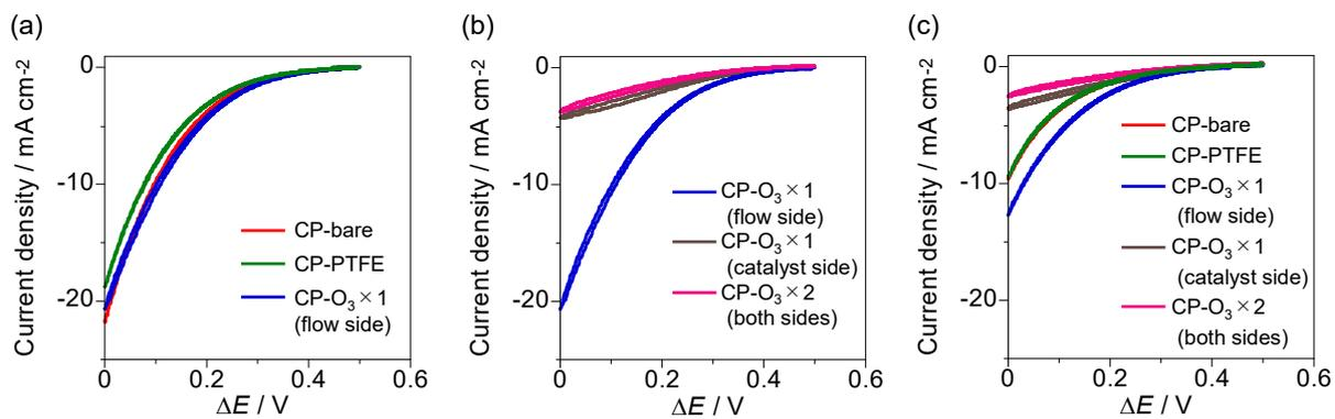
**Figure S3.** Cyclic voltammograms of the PEMFR with different GDLs: CP-bare, CP-PTFE, and CP-O<sub>3</sub> × 1 (flow side treated) (a) and various ozone-treated CP-O<sub>3</sub> (b). O<sub>2</sub> and water simultaneously flowed into the cathode at 50 and 0.50 mL min<sup>-1</sup>, respectively. Cyclic voltammograms after the reactor operation for 4 h at a fuel cell voltage of 0.10 V (c).
