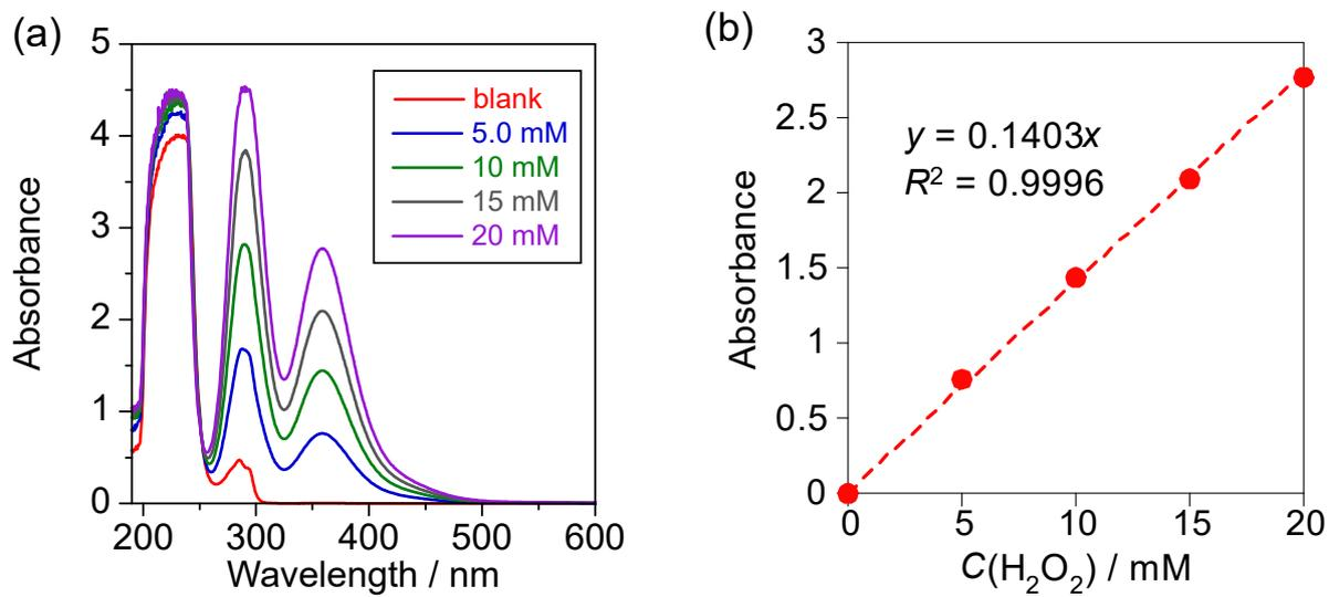
**Figure S1.** Spectrophotometric determination of H<sub>2</sub>O<sub>2</sub> in methanol by potassium iodide method:
