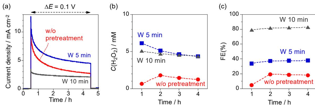
**Figure S4.** Current-time curves (a), the concentration of produced H<sub>2</sub>O<sub>2</sub> (b), and FE for H<sub>2</sub>O<sub>2</sub> (c) of the PEMFR with CP-O<sub>3</sub>×1 (catalyst side) GDL after different pretreatment with water flow at 5.0 mL min<sup>-1</sup> for 5 min (W 5 min) and 10 min (W 10 min). The reaction was performed under simultaneous flows of O<sub>2</sub> gas (50 mL min<sup>-1</sup>) and water (0.50 mL min<sup>-1</sup>).
