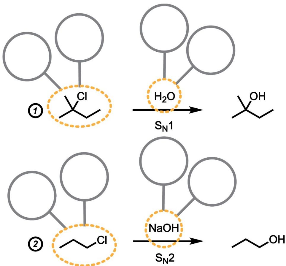
The above reactions present two contrasting reactions: One S<sub>N</sub>1 reaction and one S<sub>N</sub>2 reaction. The dotted yellow lines indicate important species in the reaction. Fill in each grey circle connected to the dotted yellow lines with a feature you can infer from each species (i.e.: strong nucleophile, primary leaving group, good leaving group, etc.). Also, please indicate why you can infer your chosen feature (i.e., why it is a good leaving group).
