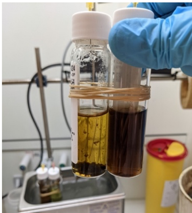
Figure S5: Digital photograph of Fe-BTC/PDA-DIP (left) and Fe-BTC/PDA (right) digested in EDTA solution.
