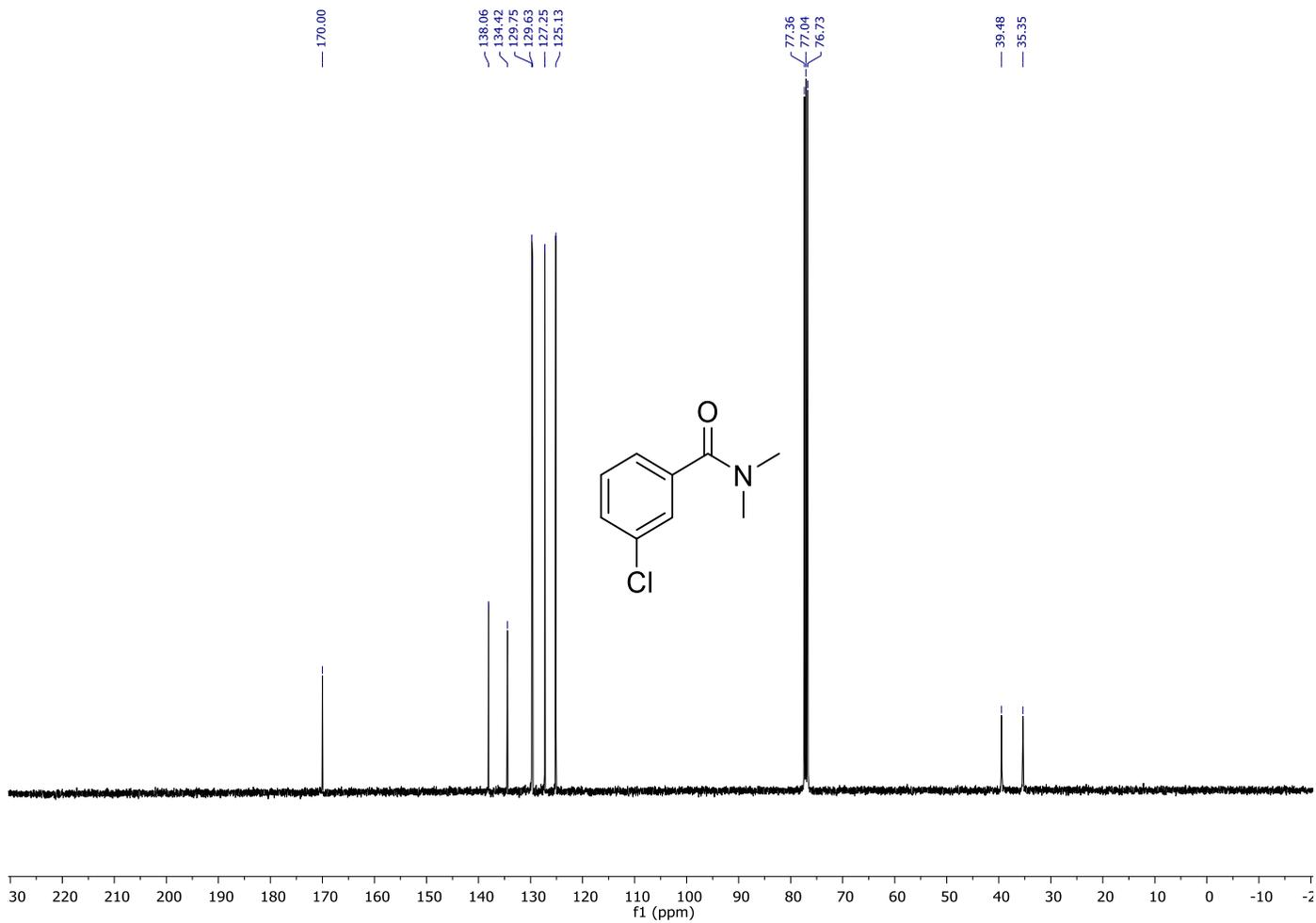
$^{13}\text{C}\{^1\text{H}\}$  NMR ( $\text{CDCl}_3$ , 101 MHz) spectrum of **1j**.
