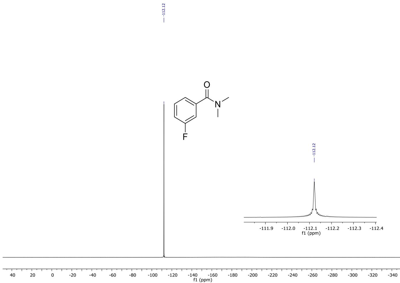
$^{19}\text{F}\{^1\text{H}\}$  NMR ( $\text{CDCl}_3$ , 376 MHz) spectrum of **1i**.
