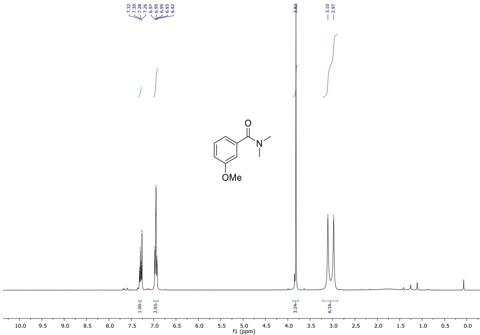
$^1\text{H}$  NMR ( $\text{CDCl}_3$ , 400 MHz) spectrum of **1**.
