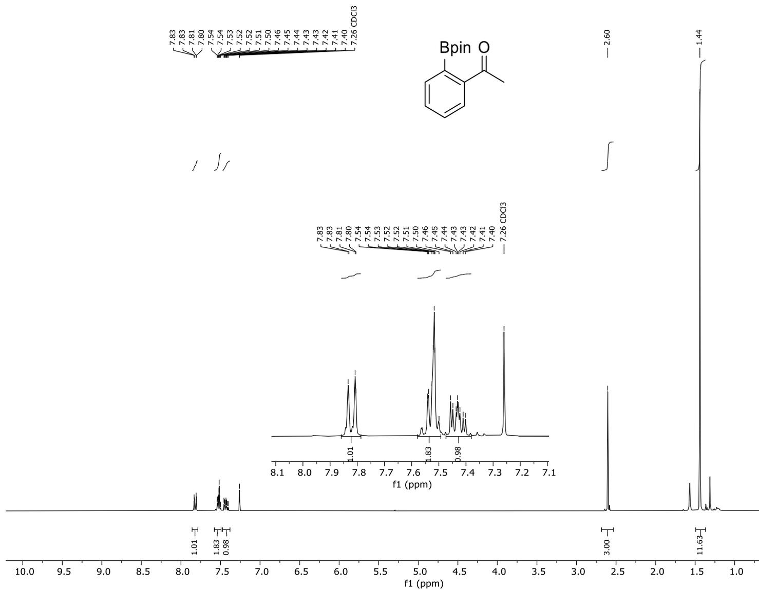
**<sup>1</sup>H NMR (CDCl<sub>3</sub>, 400 MHz) spectrum of 2p.**
