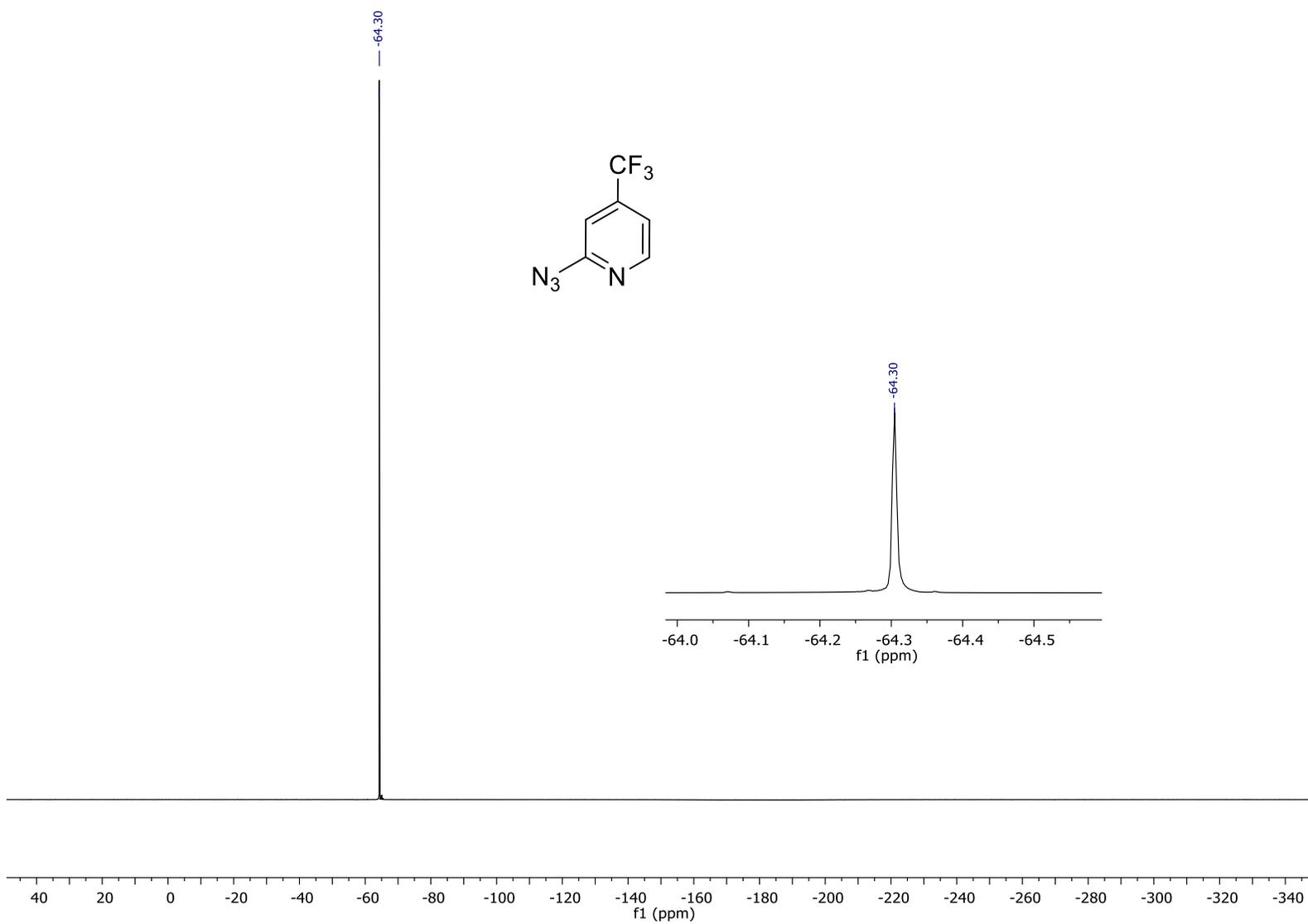
$^{19}\text{F}\{^1\text{H}\}$  NMR ( $\text{CDCl}_3$ , 376 MHz) spectrum of 2-azido-4-(trifluoromethyl)pyridine (AP6).
