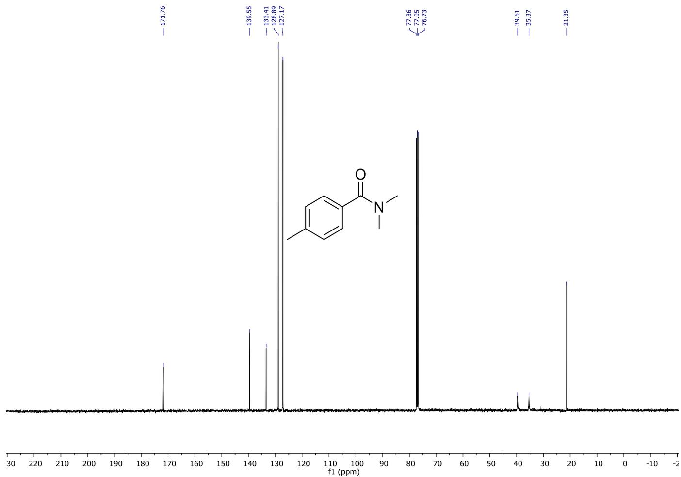
$^{13}\text{C}\{^1\text{H}\}$  NMR ( $\text{CDCl}_3$ , 101 MHz) spectrum of **1n**.
