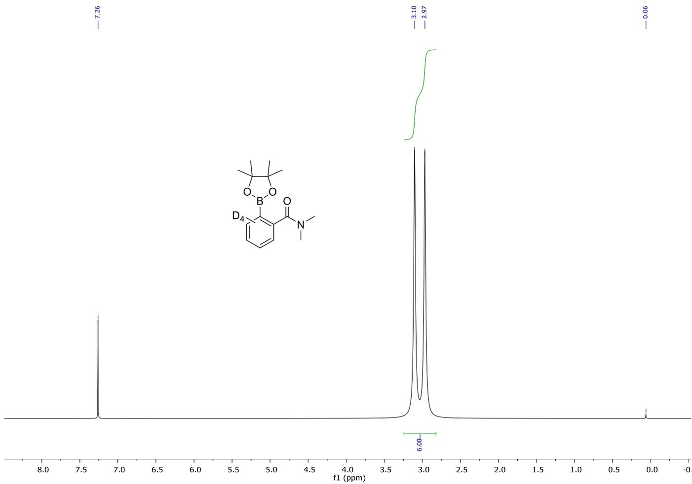
$^1\text{H}$  NMR ( $\text{CDCl}_3$ , 400 MHz) spectrum of 2-(4,4,5,5-tetramethyl-1,3,2-dioxaborolan-2-yl)-3,4,5,6- $\text{D}_5$ - $N,N'$ -dimethylbenzamide **1a-d<sub>5</sub>**.
