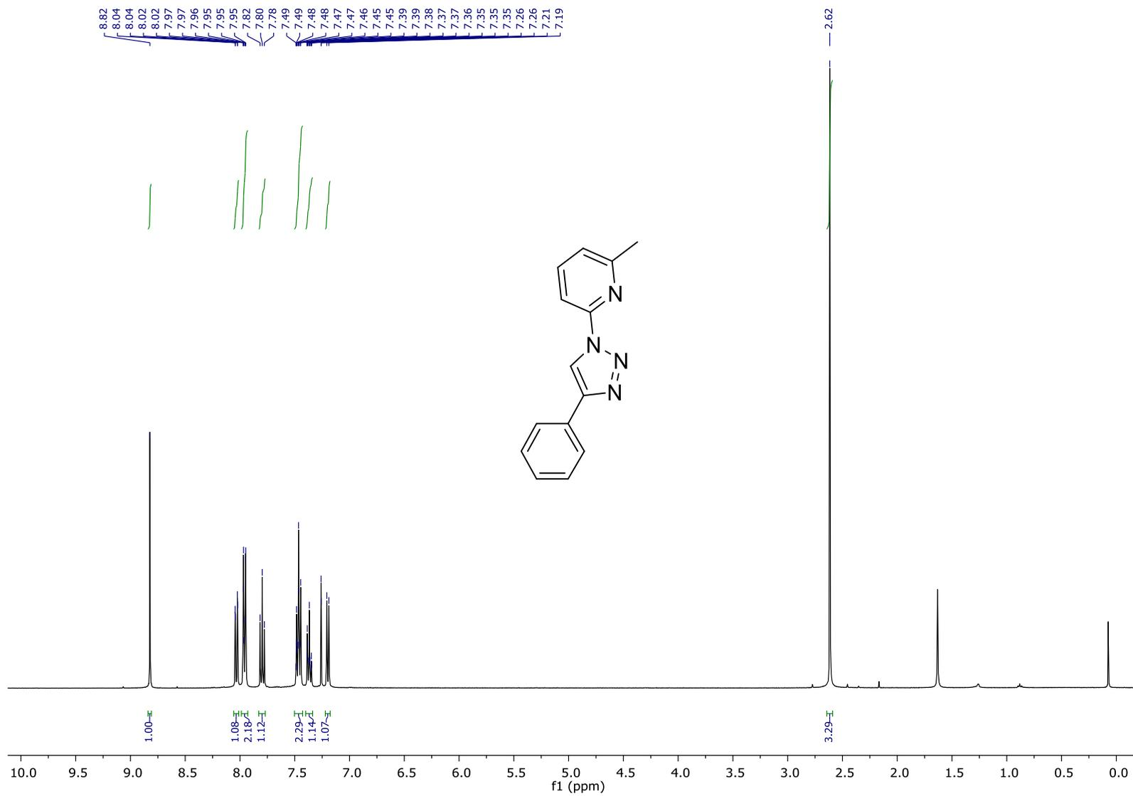
$^1\text{H}$  NMR ( $\text{CDCl}_3$ , 400 MHz) spectrum of **L4\***.
