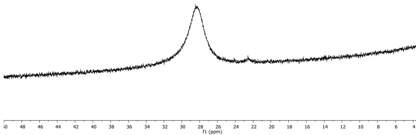
$^{11}\text{B}\{^1\text{H}\}$  NMR ( $\text{CDCl}_3$ , 128 MHz) spectrum spectrum of **2n**.
