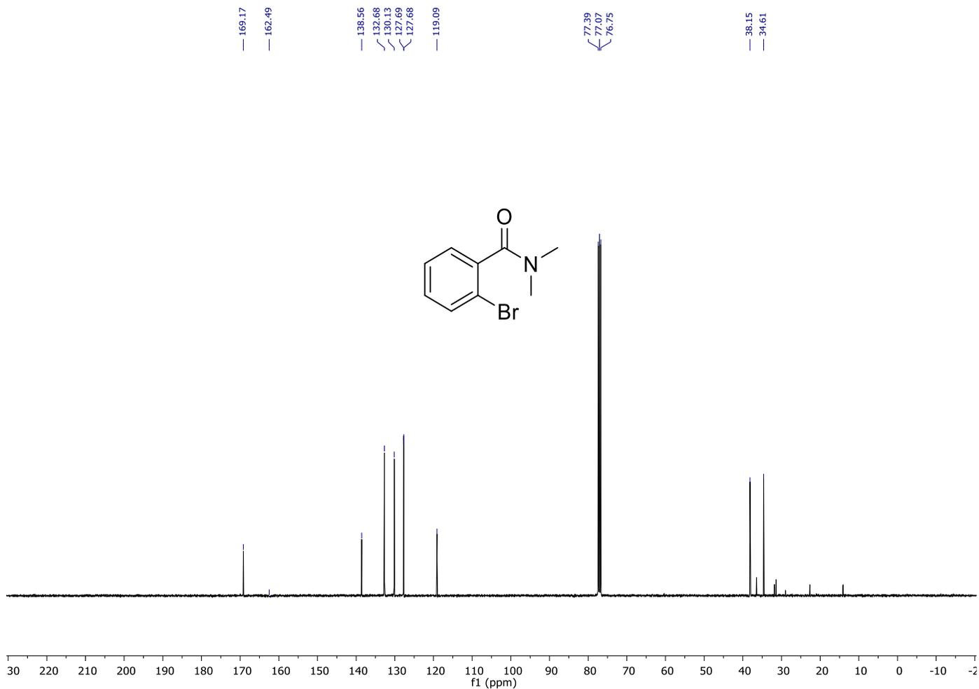
$^{13}\text{C}\{^1\text{H}\}$  NMR ( $\text{CDCl}_3$ , 101 MHz) spectrum of **1h**.
