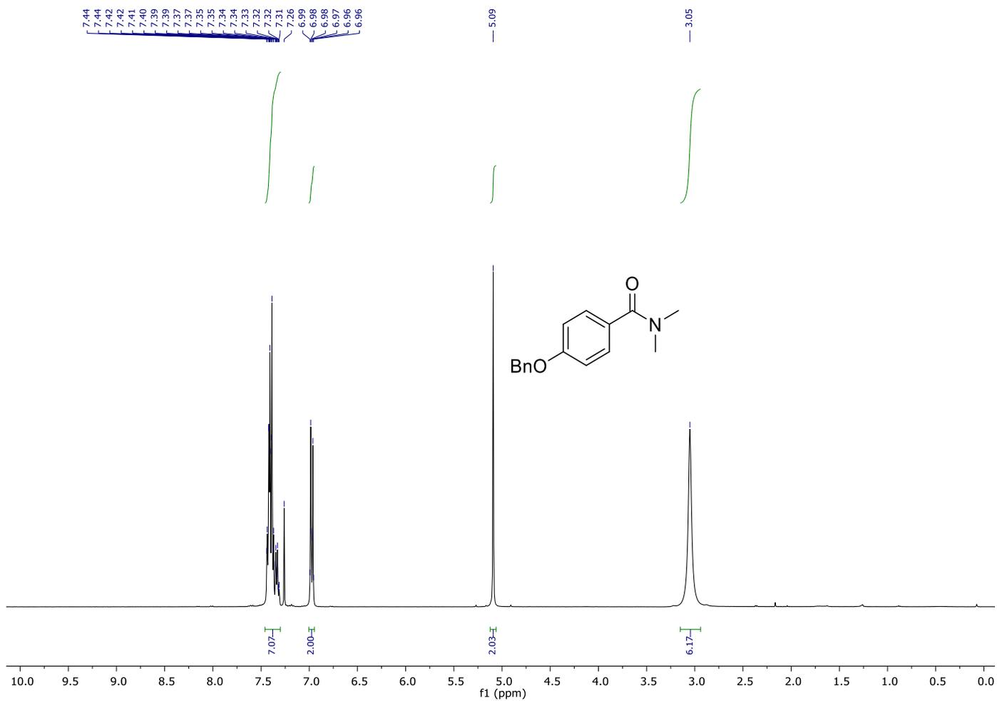
$^1\text{H}$  NMR ( $\text{CDCl}_3$ , 400 MHz) spectrum of **1o**.
