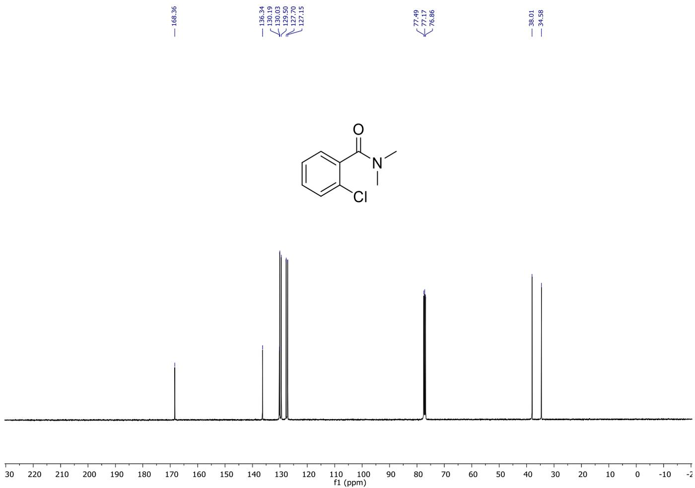
$^{13}\text{C}\{^1\text{H}\}$  NMR ( $\text{CDCl}_3$ , 101 MHz) spectrum of **1g**.
