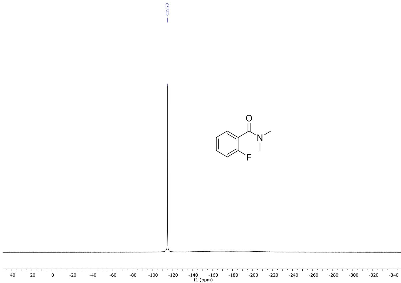
$^{19}\text{F}\{^1\text{H}\}$  NMR ( $\text{CDCl}_3$ , 376 MHz) spectrum of **1f**.
