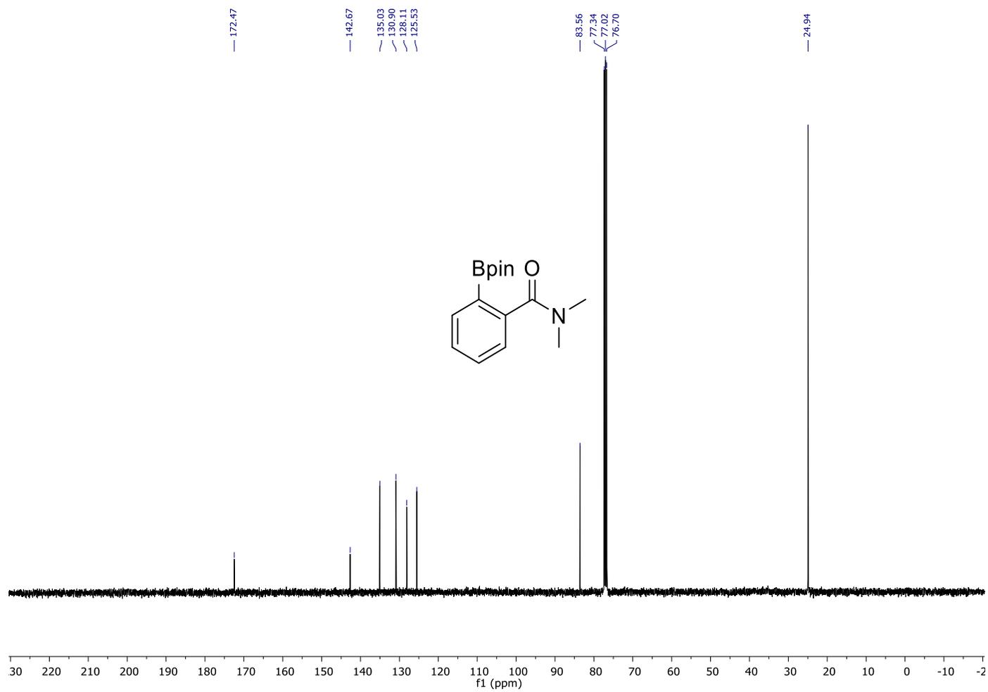
$^{13}\text{C}\{^1\text{H}\}$  NMR ( $\text{CDCl}_3$ , 101 MHz) spectrum of **2a**.
