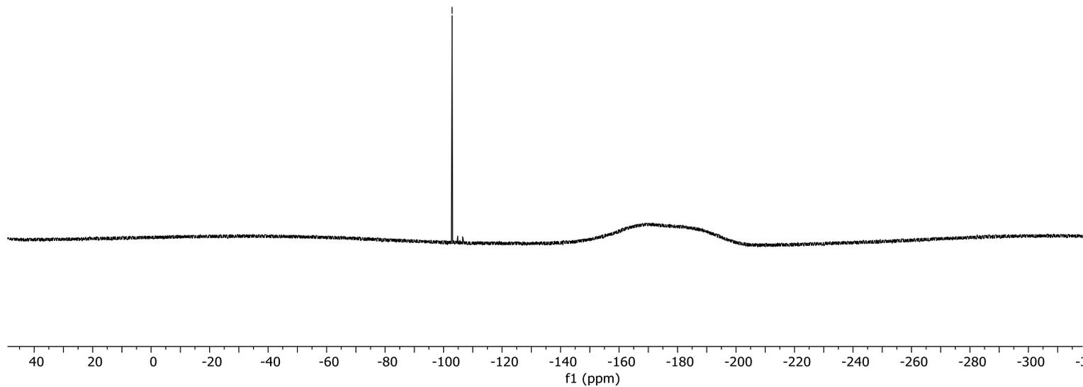
$^{19}\text{F}\{^1\text{H}\}$  NMR ( $\text{CDCl}_3$ , 376 MHz) spectrum of **2i**.
