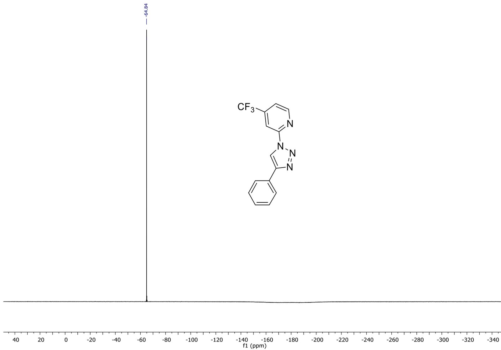
$^{19}\text{F}\{^1\text{H}\}$  NMR ( $\text{CDCl}_3$ , 376 MHz) spectrum of **L6\***.
