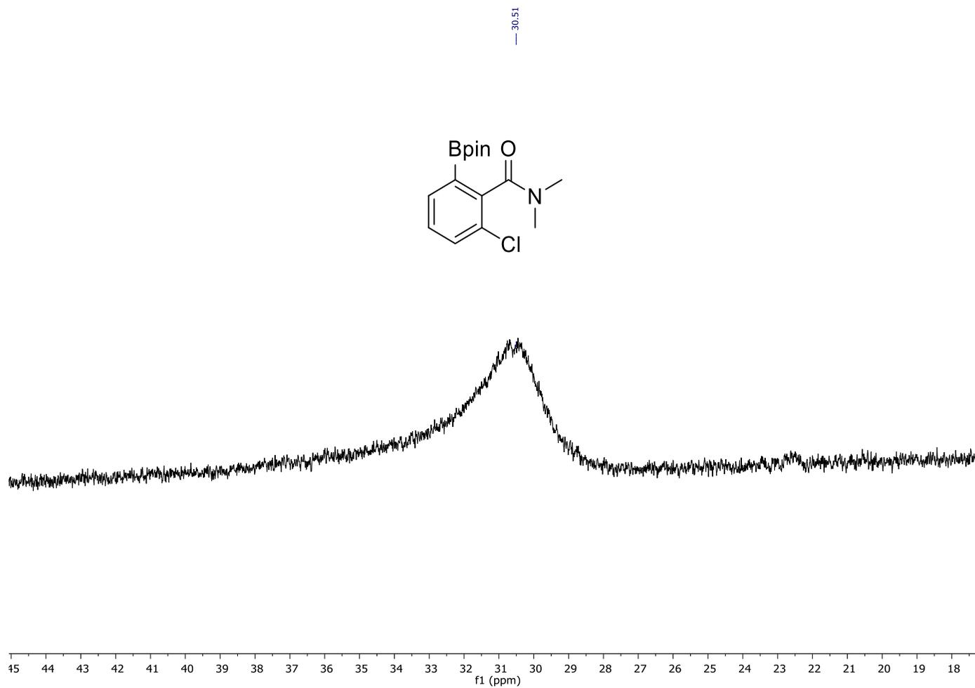
$^{11}\text{B}\{^1\text{H}\}$  NMR ( $\text{CDCl}_3$ , 128 MHz) spectrum spectrum of **2g**.
