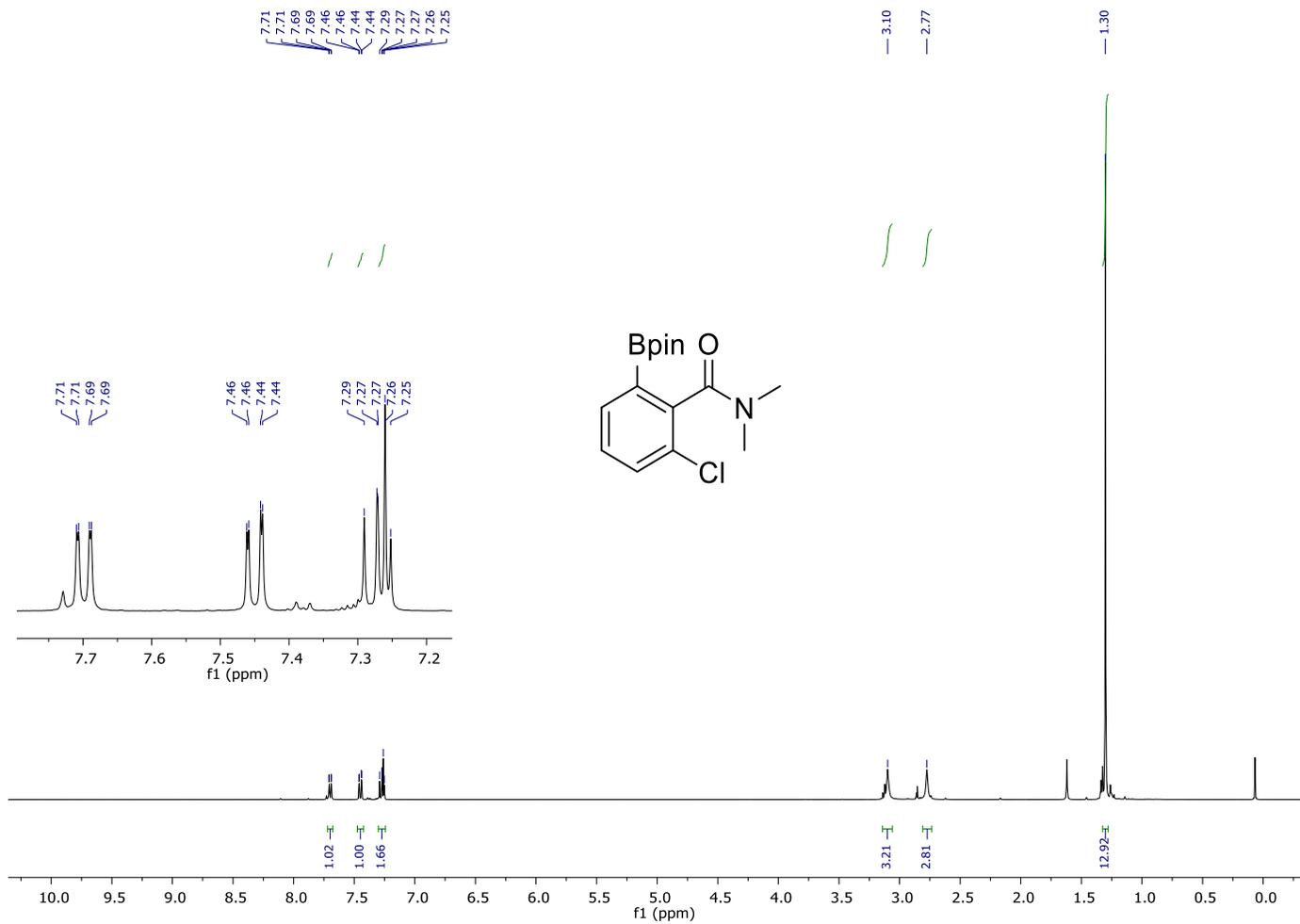
$^1\text{H}$  NMR ( $\text{CDCl}_3$ , 400 MHz) spectrum of **2g**.
