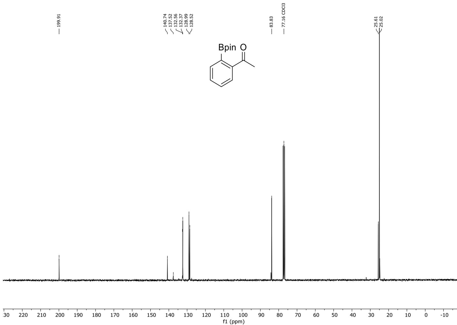
$^{13}\text{C}\{^1\text{H}\}$  NMR (CDCl<sub>3</sub>, 101 MHz) spectrum of 2p.
