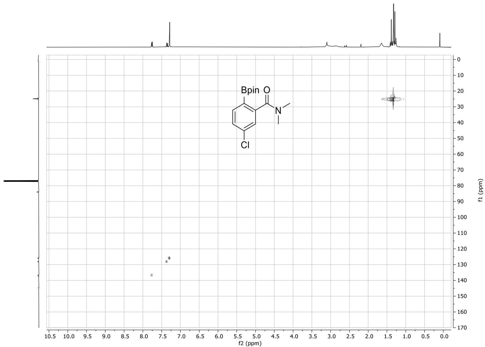
$^1\text{H}$ - $^{13}\text{C}$  HSQC NMR ( $\text{CDCl}_3$ ) spectrum of **2j**.
