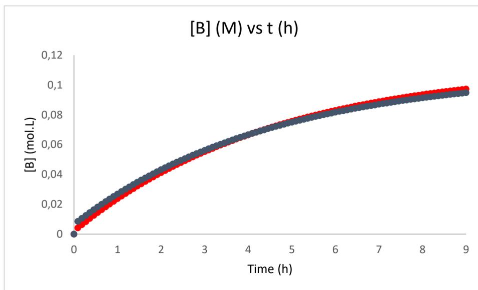
**Summary of kinetic profile:** The kinetic profiles are plotted as follow: N,N'-dimethylbenzamide kinetic profile in red and 2,3,4,5,6-d<sub>5</sub>-N,N'-dimethylbenzamide kinetic profile in blue.
