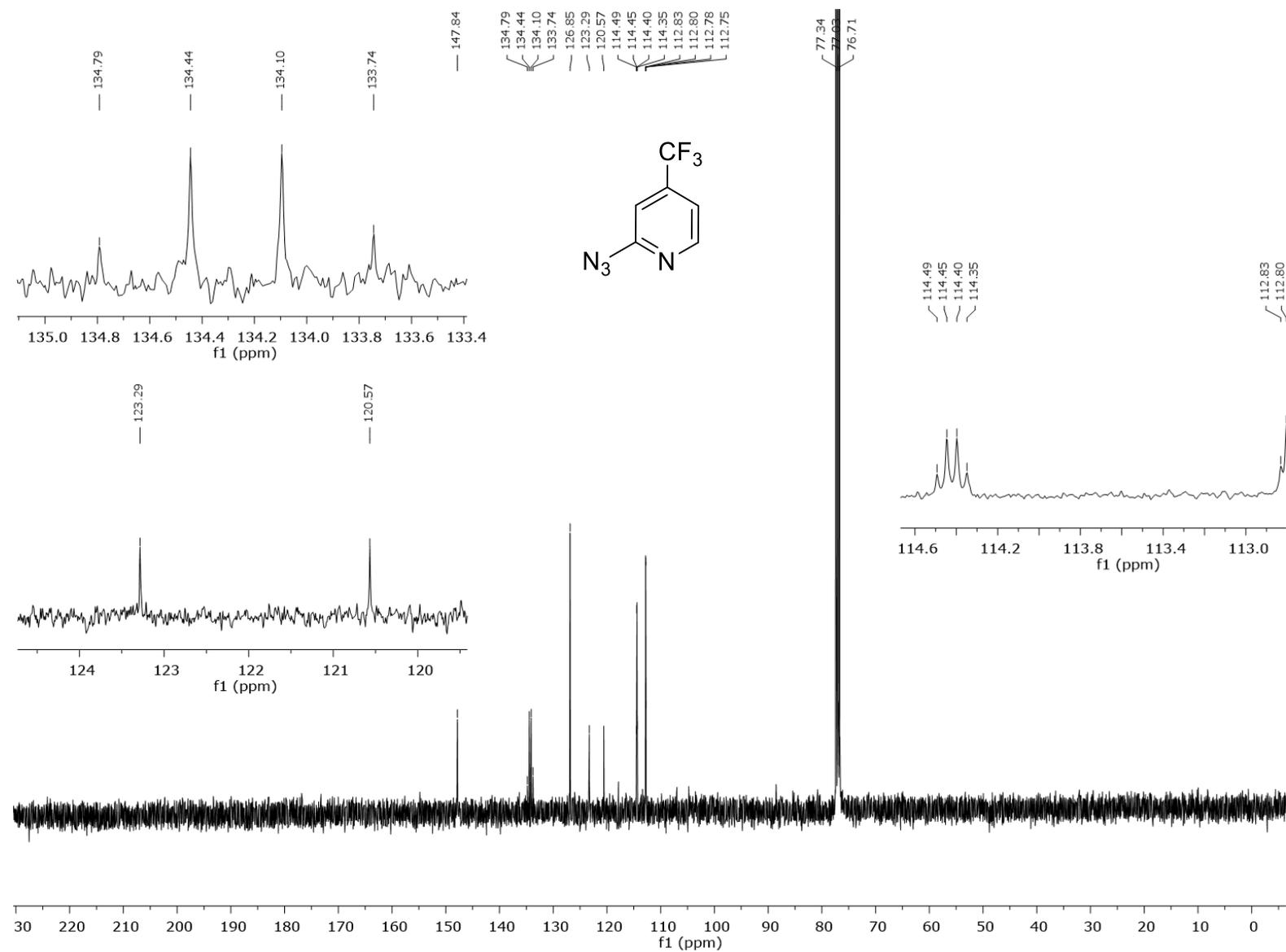
$^{13}\text{C}\{^1\text{H}\}$  NMR ( $\text{CDCl}_3$ , 101 MHz) spectrum of 2-azido-4-trifluoromethylpyridine (AP6).
