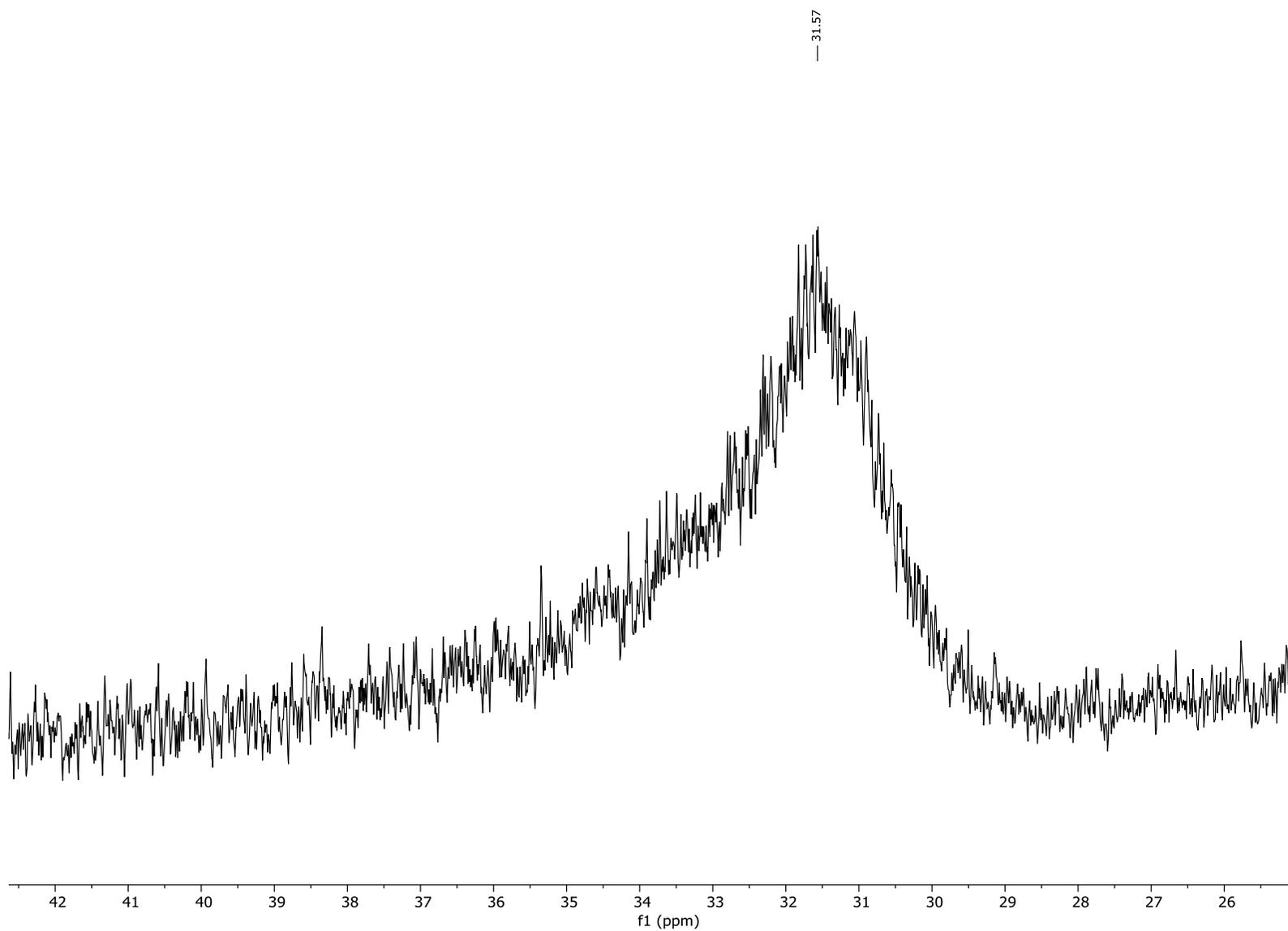
$^{11}\text{B}\{^1\text{H}\}$  NMR ( $\text{CDCl}_3$ , 128 MHz) spectrum spectrum of **2p**.
