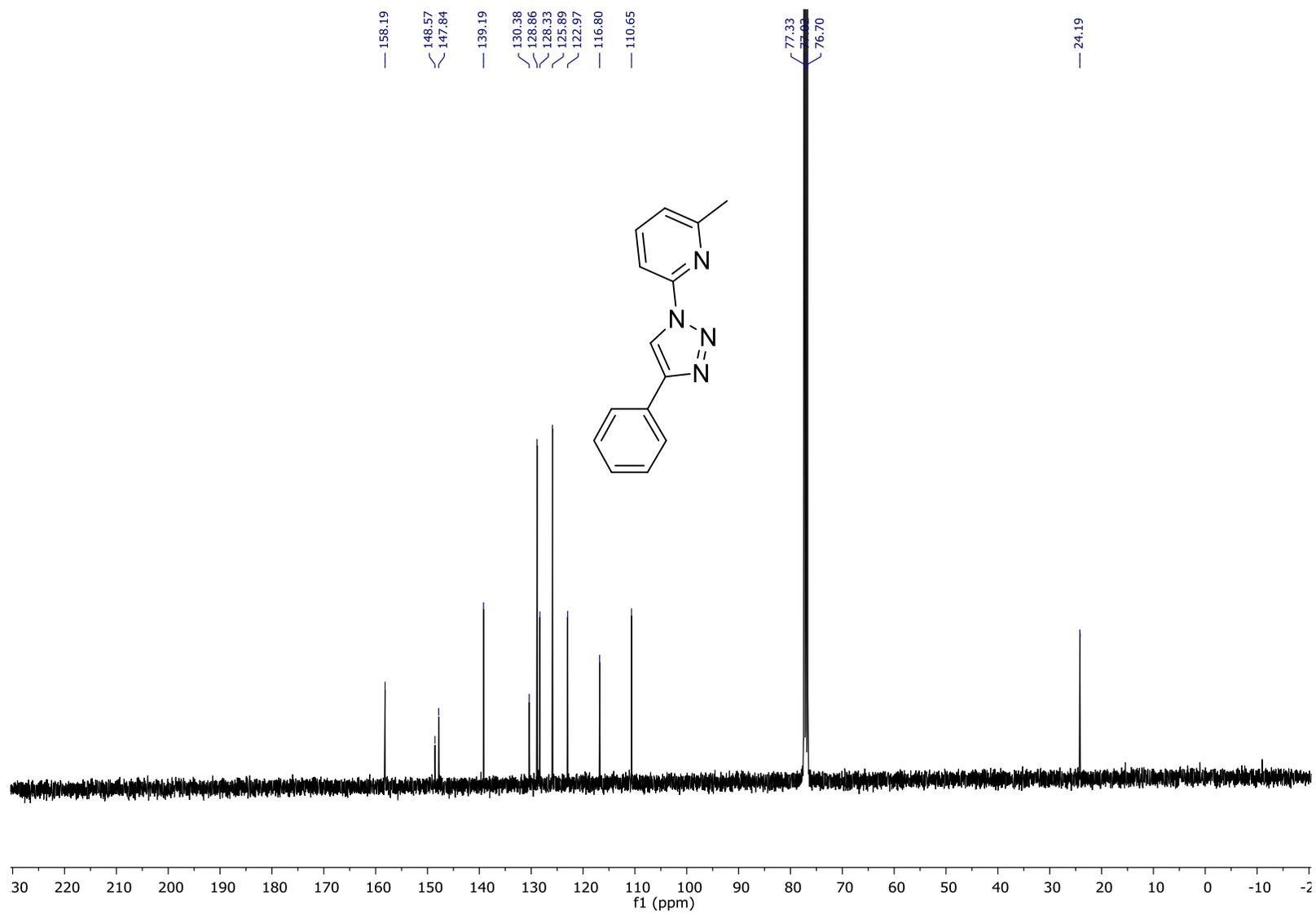
$^{13}\text{C}\{^1\text{H}\}$  NMR ( $\text{CDCl}_3$ , 101 MHz) spectrum of **L4\***.
