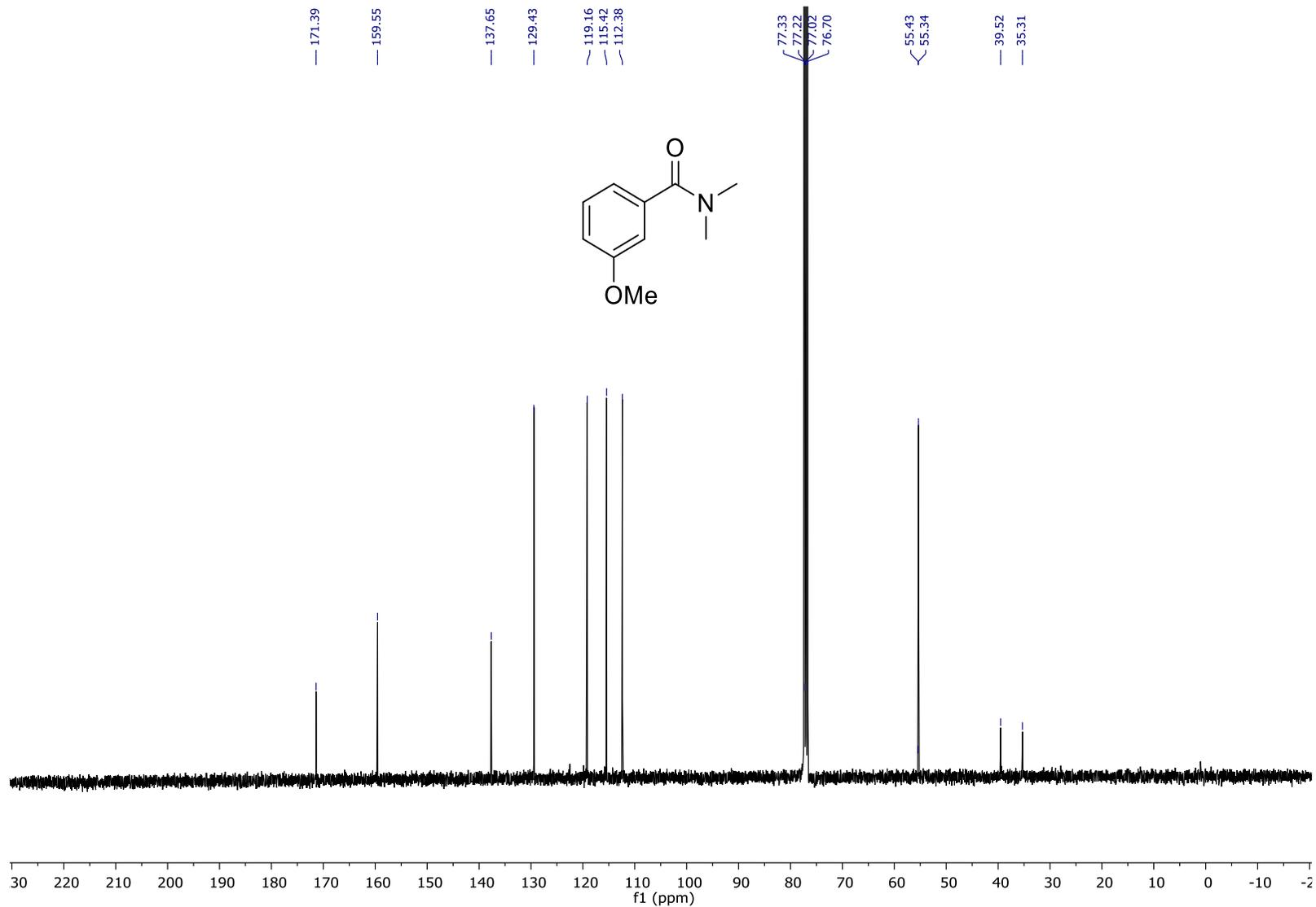
$^{13}\text{C}\{^1\text{H}\}$  NMR ( $\text{CDCl}_3$ , 101 MHz) spectrum of **1I**.
