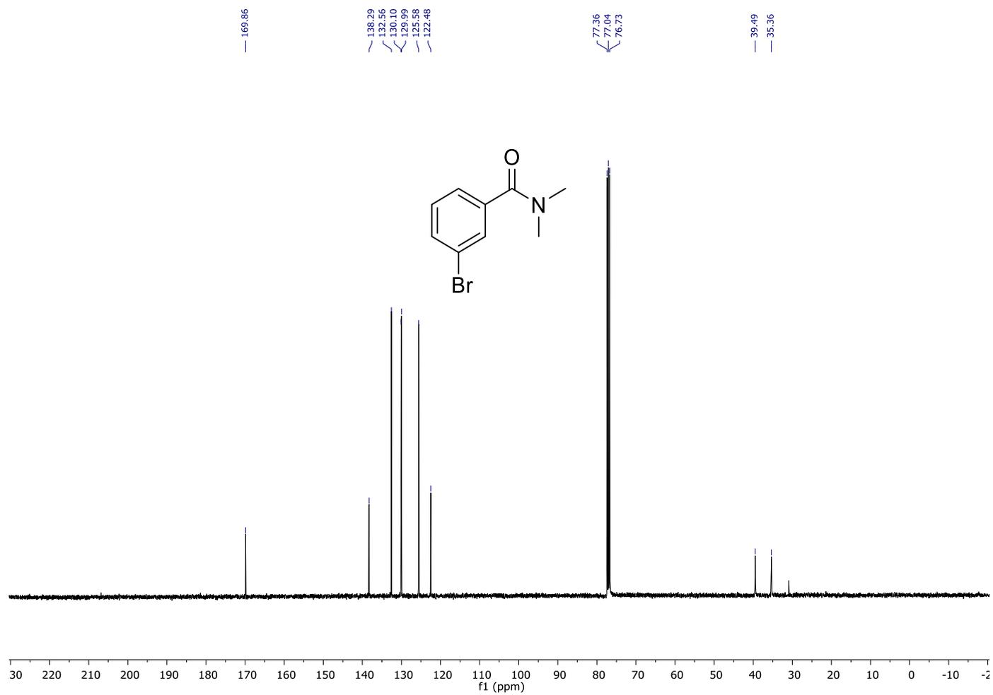
$^{13}\text{C}\{^1\text{H}\}$  NMR ( $\text{CDCl}_3$ , 101 MHz) spectrum of **1k**
