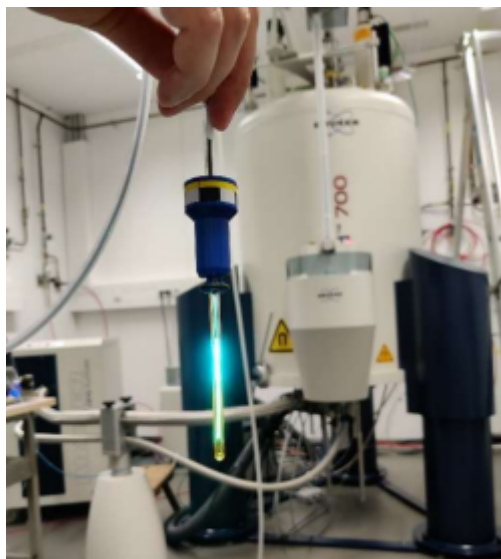
Figure S45. Visual presentation of the in-situ NMR irradiation set up: An NMR sample with a quartz-glass insert and an optical fibre. 5
