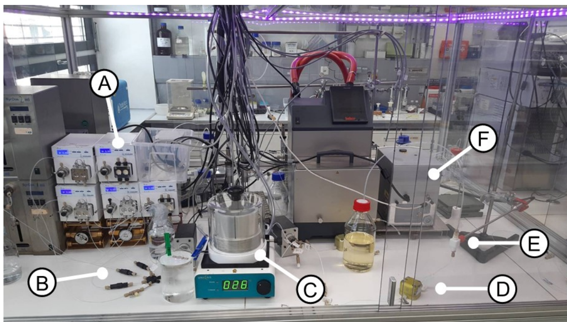
Figure S9. Photograph of the experimental setup in the laboratory. A: HPLC pumps, B: cartridge BPRs and mixing unit (7-port connector), C: Uniqlis coil heater, D: reactor BPR, E: FTIR probe inside in-house built flow cell, F: FTIR instrument.
