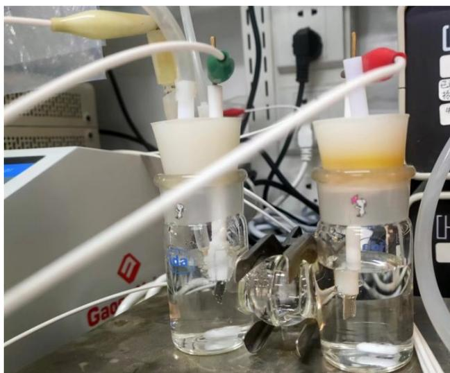
**Fig. S16.** Photo of the used H-cell.
