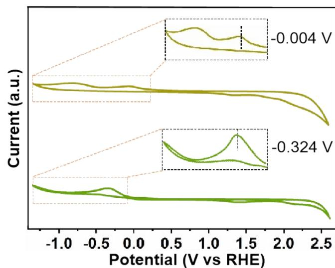
**Figure S10** Cyclic voltammograms of *d-S<sub>T</sub>* (green line) and *d-C<sub>T</sub>* (yellow line) containing 0.1 M Tetrabutylammonium perchlorate. Scan rate: 100 mV/s
