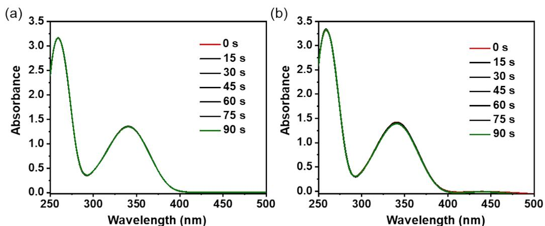
**Figure S12** Photocatalytic oxidation for 90 s in air condition recorded by absorption spectra. (a) NADPH alone (50 μM); (b) *d-C<sub>T</sub>* (10 μM) + NADPH (50 μM).
