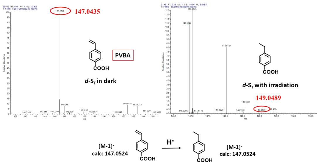
**Figure S11** HRMS analysis of *d-S<sub>T</sub>* containing PVBA (10 mM) under NIR light irradiation for 1 min.
