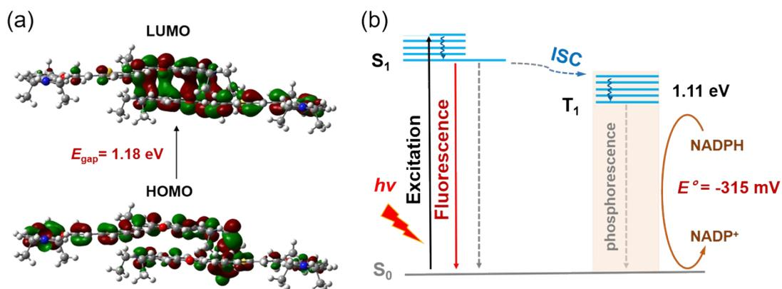
**Figure S14** Frontier molecular orbital distributions and energy levels of  $d-S_T$  calculated using density functional theory (DFT) method at the B3LYP/6-31G (d, p) level.
