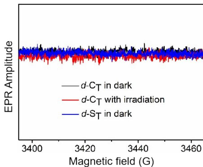
**Figure S9** Electron spin resonance spectra of DMPO/ $d-S_T$  in dark (blue) and DMPO/ $d-C_T$  in 10 % DMSO- $H_2O$  in dark (black) or light for 1 min (red).
