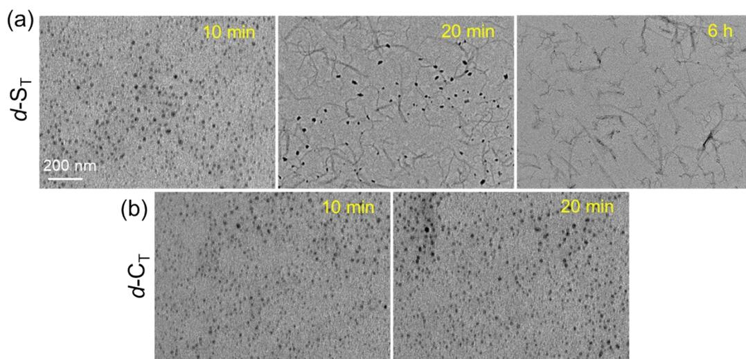
**Figure S7** TEM images of assembled *d-S<sub>T</sub>* (a) and *d-C<sub>T</sub>* (b) in deionized water at different time points.
