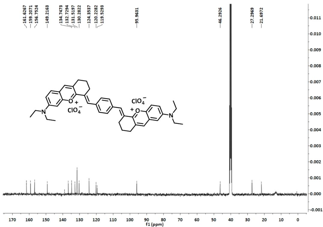
Figure S5  $^{13}C$  NMR spectrum of  $d-C_T$  in DMSO at room temperature.
