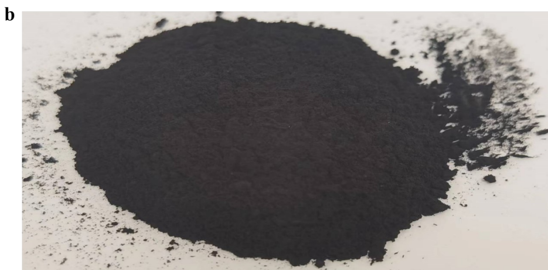
Figure S2. Image of R-C-dots before vacuum filtration. (a) The beaker used for the reaction is lined with a large amount of R-C-dots powder, as well as (b) a solid powder of R-C-dots obtained by vacuum filtration.
