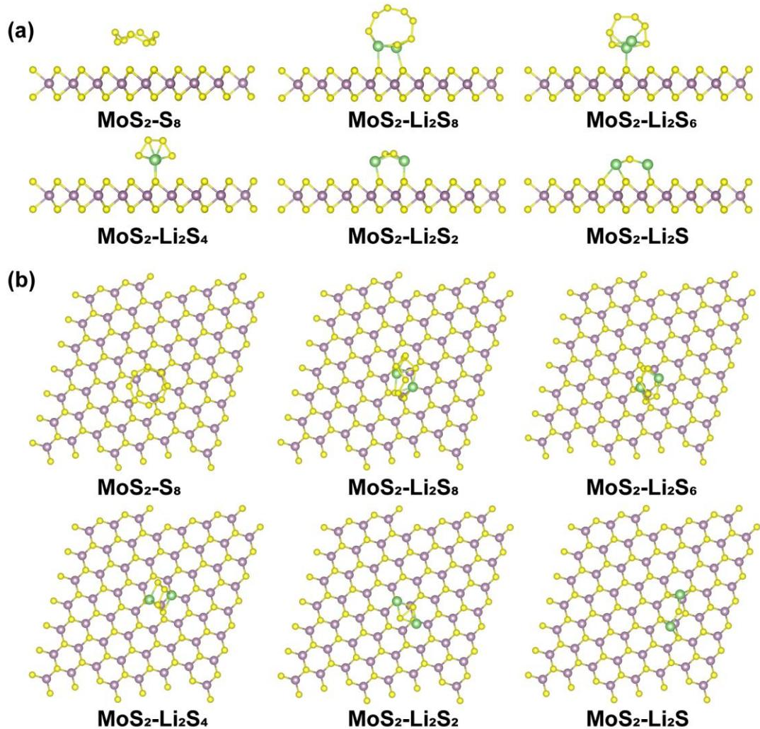
Figure S12 Side (a) and top (b) views of the adsorption configurations of LiPSs on MoS<sub>2</sub> (002).
