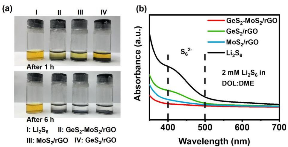
Figure S14 (a) Optical images of  $\text{Li}_2\text{S}_6$  solutions after 1 h and 6 h adsorption, respectively; (b) UV-Vis spectra of  $\text{Li}_2\text{S}_6$  solutions after exposure to different catalysts.
