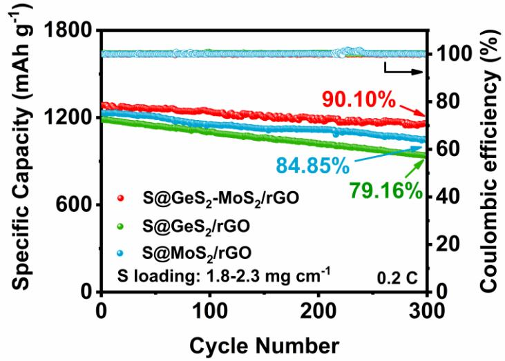
Figure S15 Cycling life of different electrodes at 0.2 C over 300 cycles.
