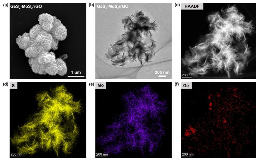
Figure S5 (a) SEM image of  $\text{GeS}_2\text{-MoS}_2/\text{rGO}$ ; (b) TEM image of  $\text{GeS}_2\text{-MoS}_2/\text{rGO}$ ; (c-f) EDX images of  $\text{GeS}_2\text{-MoS}_2/\text{rGO}$ .
