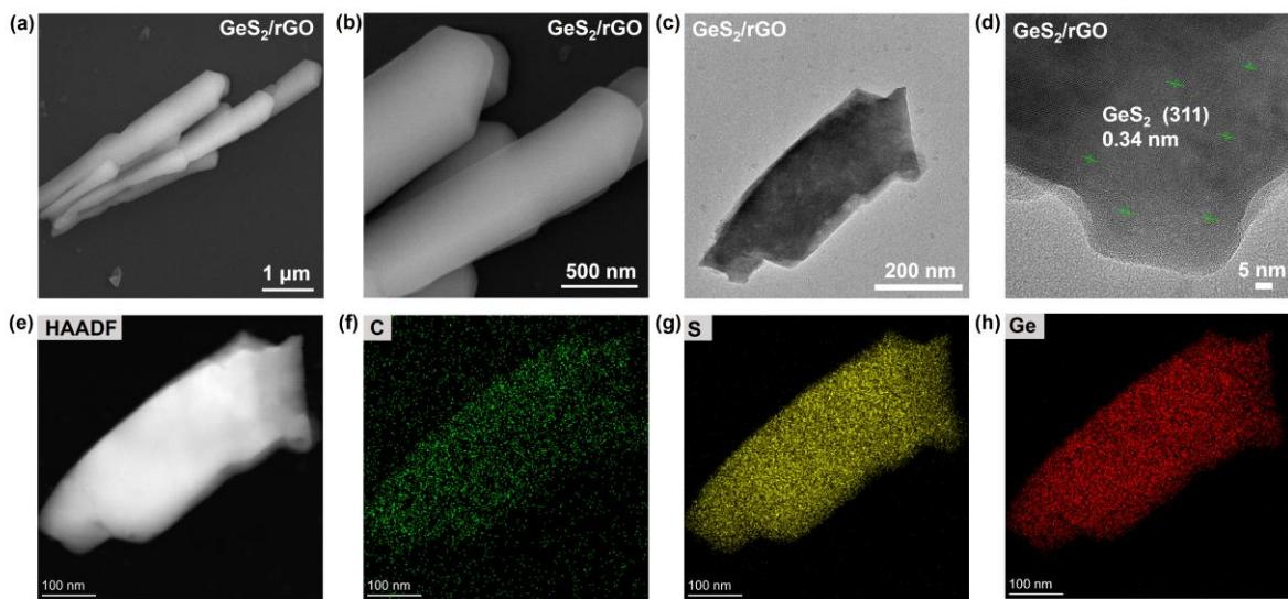
Figure S8 (a-b) SEM images of the GeS<sub>2</sub>/rGO; (c-d) TEM and HRTEM images of the GeS<sub>2</sub>/rGO; (e-h) EDX images of the GeS<sub>2</sub>/rGO.
