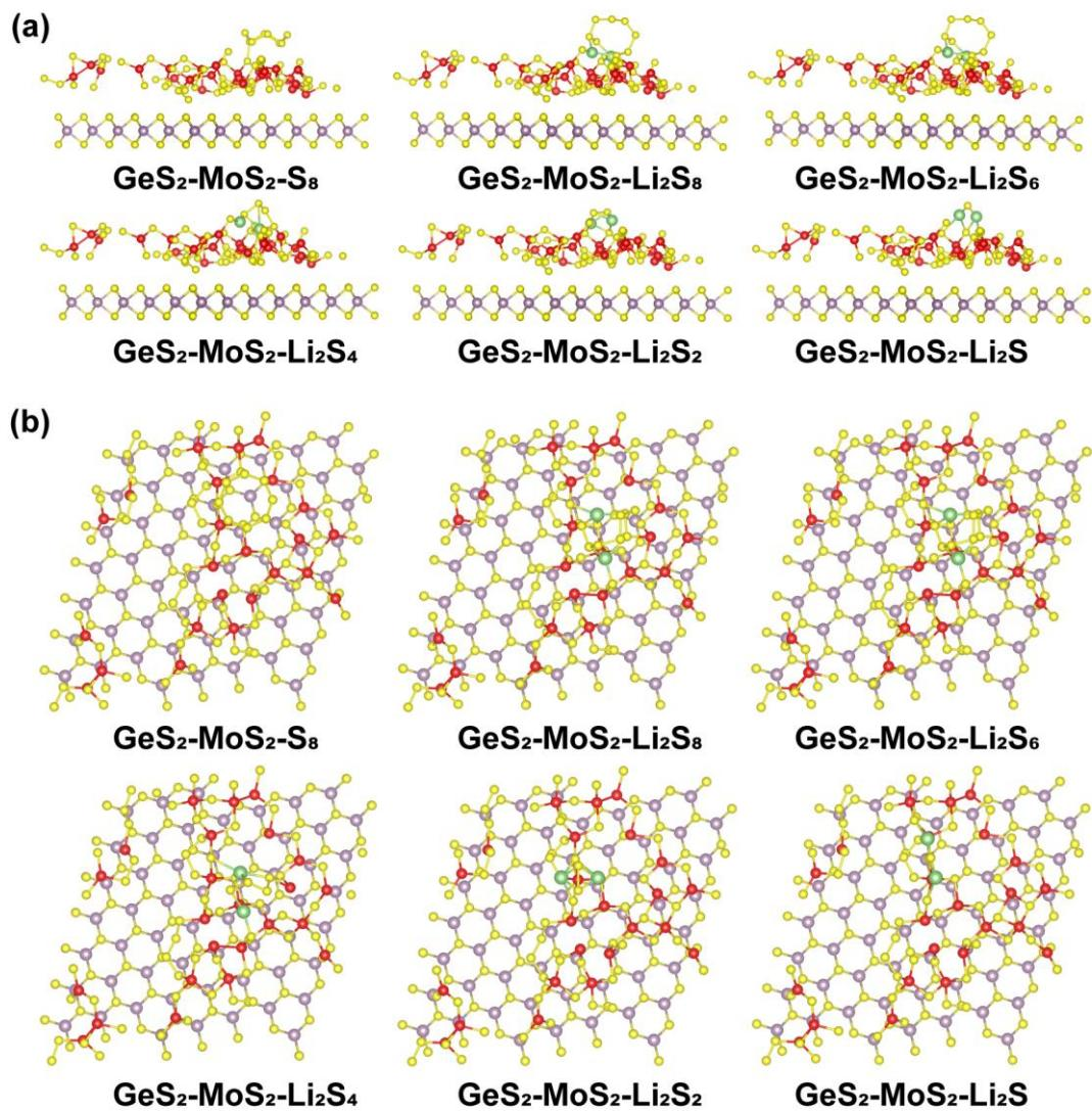
Figure S11 Side (a) and top (b) views of the adsorption configurations of LiPSs on the GeS<sub>2</sub>-MoS<sub>2</sub> heterostructure.
