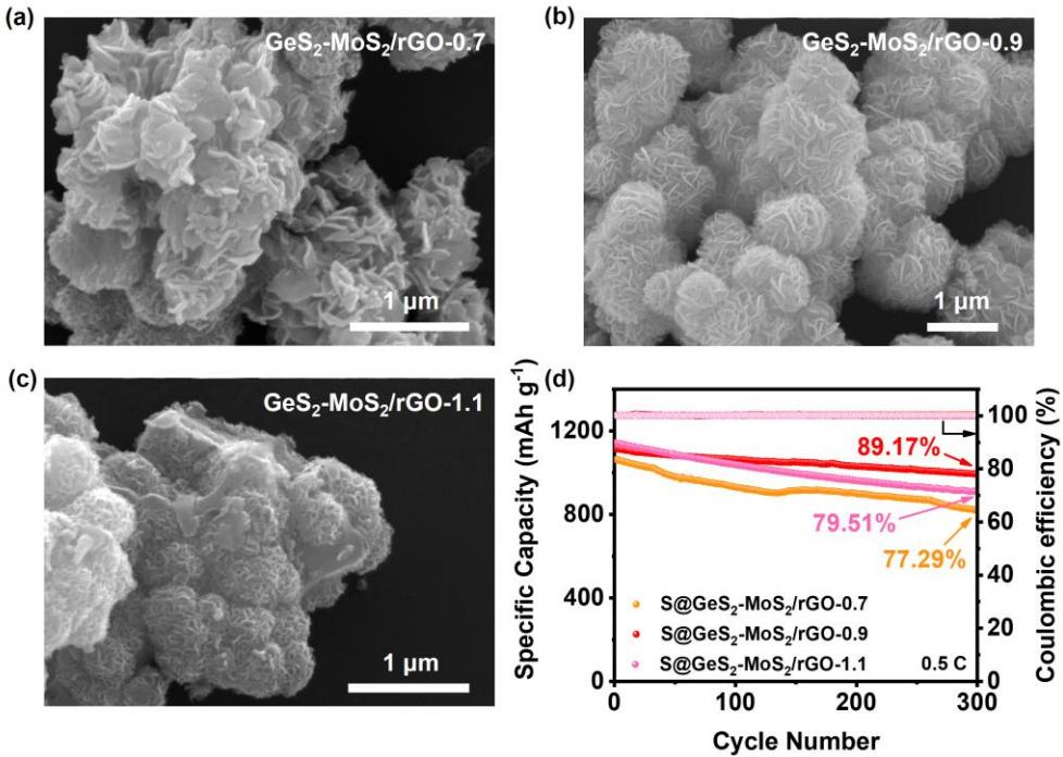
Figure S4 (a-c) SEM images of  $\text{GeS}_2\text{-MoS}_2/\text{rGO}$  with different ratios; (d) Cycling capacity of  $\text{GeS}_2\text{-MoS}_2/\text{rGO}$  with different ratios at 0.5 C over 300 cycles.
