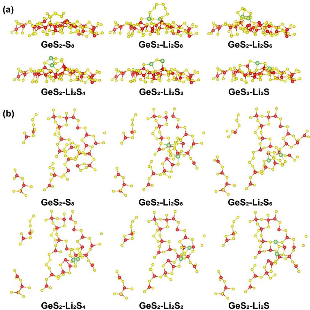
Figure S13 Side (a) and top (b) views of the adsorption configurations of LiPSs on GeS<sub>2</sub> (311).
