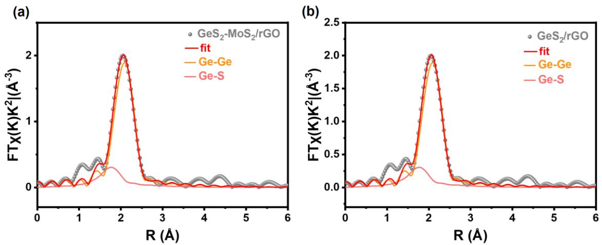
Figure S3 (a-b) The fitted R-space of EXAFS analysis of Ge in  $\text{GeS}_2\text{-MoS}_2/\text{rGO}$  and  $\text{GeS}_2/\text{rGO}$ , respectively.
