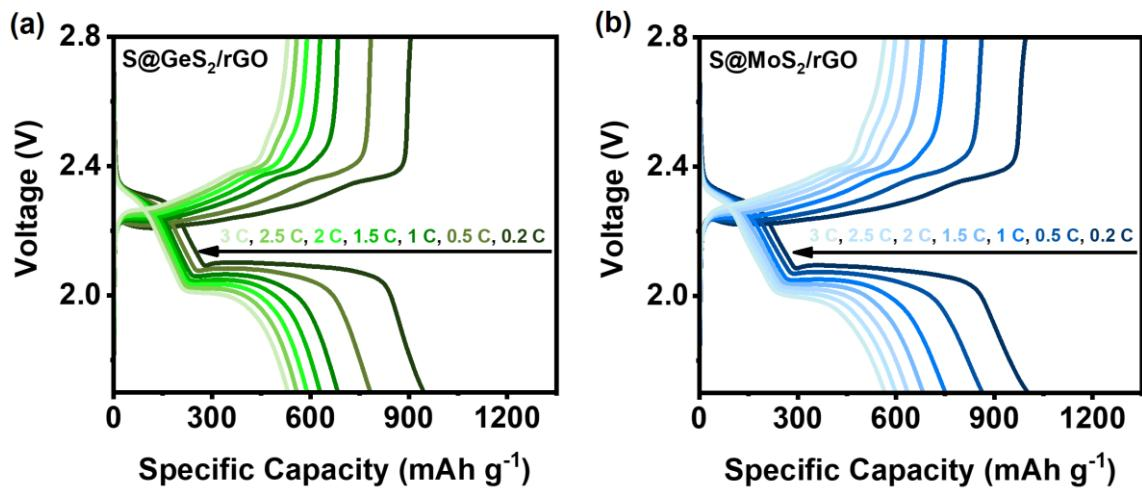
Figure S16 (a-b) Galvanostatic discharge/charge profiles of S@GeS<sub>2</sub>/rGO and S@MoS<sub>2</sub>/rGO with various current densities, respectively.
