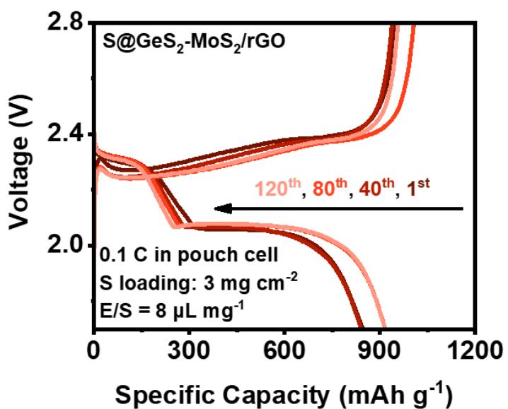
Figure S17 Galvanostatic discharge/charge profiles of pouch cell with the S@GeS<sub>2</sub>-MoS<sub>2</sub>/rGO cathode.
