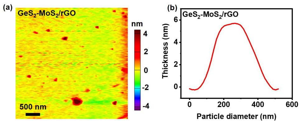
Figure S6 (a) AFM image and corresponding (b) particle size and thickness distribution of  $\text{GeS}_2\text{-MoS}_2/\text{rGO}$ . The particle distribution of  $\text{GeS}_2\text{-MoS}_2/\text{rGO}$  is 100-500 nm with a thickness of about 6 nm.
