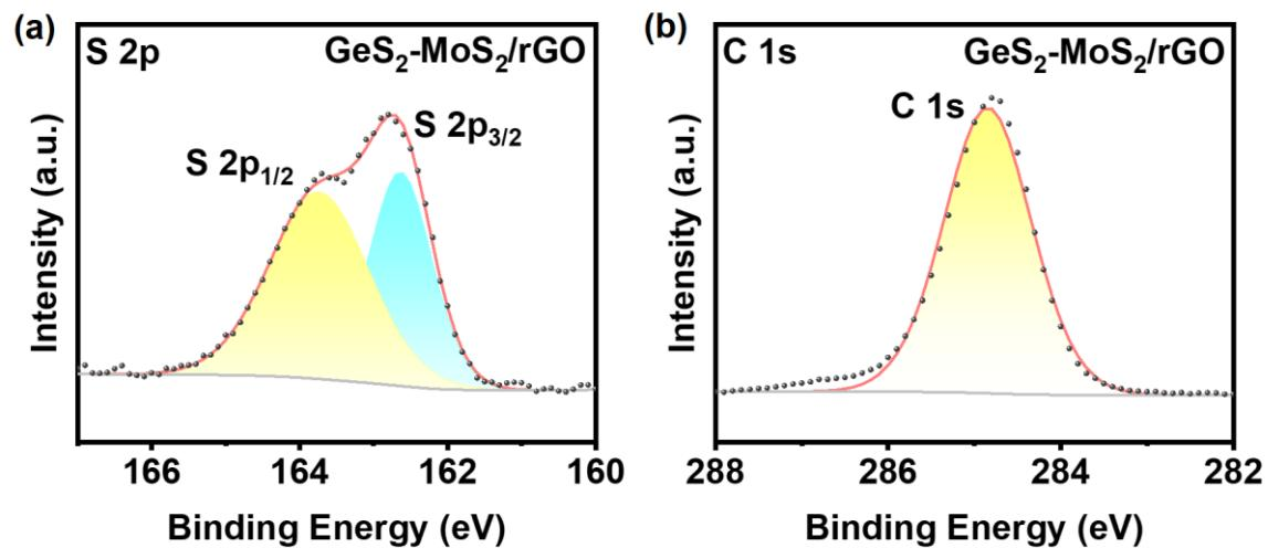
Figure S1 (a-b) High-resolution S 2p and C 1s XPS spectra of GeS<sub>2</sub>-MoS<sub>2</sub>/rGO, respectively.
