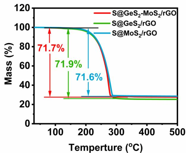
Figure S9 TG analyses of S@GeS<sub>2</sub>-MoS<sub>2</sub>/rGO, S@GeS<sub>2</sub>/rGO and S@MoS<sub>2</sub>/rGO.
