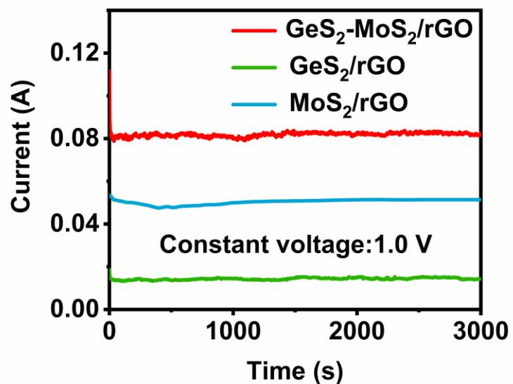
Figure S2 Electronic conductivity of GeS<sub>2</sub>-MoS<sub>2</sub>/rGO heterostructure, GeS<sub>2</sub>/rGO, and MoS<sub>2</sub>/rGO under constant voltage of 1.0 V.
